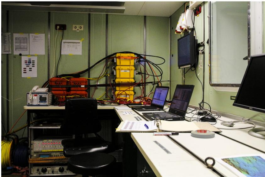
Fig. 6.3: Recording system used during PS104 seismic profiling.
