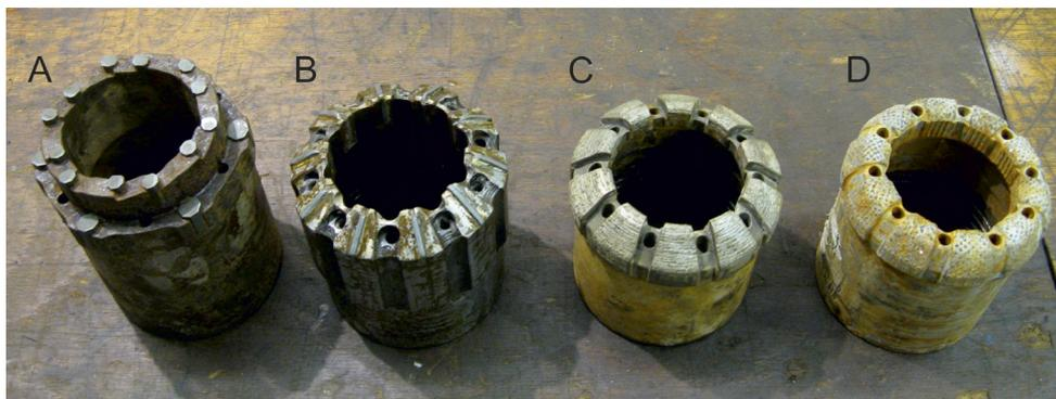
Fig. 3.3: MeBo70 drill bits used during PS104: (A) two step tungsten carbide bit; (B) conical tungsten carbide bit; (C) Diamond impregnated bit; (D) surface set diamond bit.
