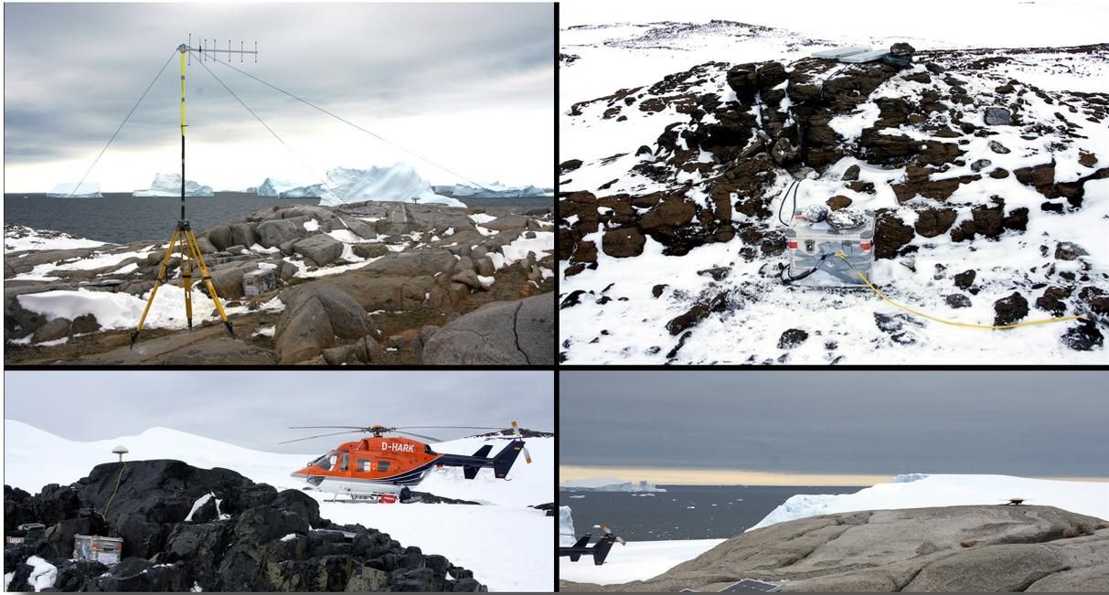
*Fig. 9.2: GPS sites on bedrock. Clockwise from upper left: Backer Islands North (BAC1), Mt. Manthe (MANT), Backer Islands South (PIG2), Clark Island (CLI1). The GPS antenna is always fixed directly to the bedrock by means of a special bolt. Solar panels provide power to charge the batteries, which are placed together with the GPS receiver within the Zarges aluminium box.*
