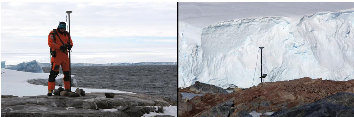
*Fig. 9.3: GPS real-time kinematic (RTK). The antenna is mounted on a special rod of defined length that enables to marking the location to be measured. The receiver is carried in a special bag. Left: Suchland Islands (site SU01), right: Molar Islands (site FE01)*
