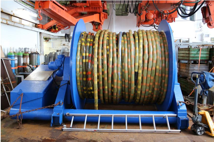
Fig. 6.2: Winch with 600 m long analogue streamer
