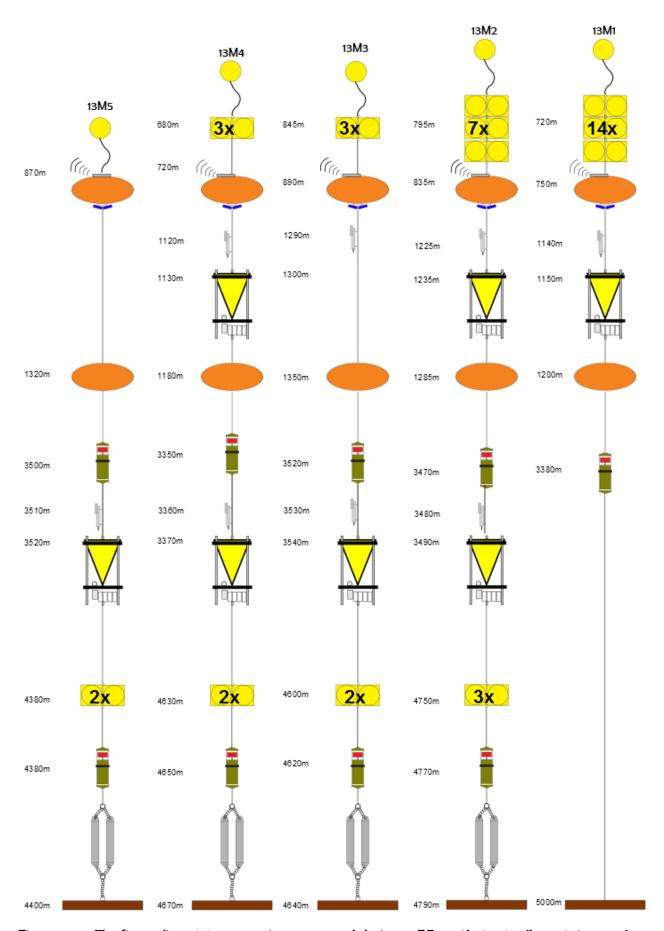
Figure 5.7.9. The five sediment-trap moorings recovered during 64PE378, that actually contain samples.
