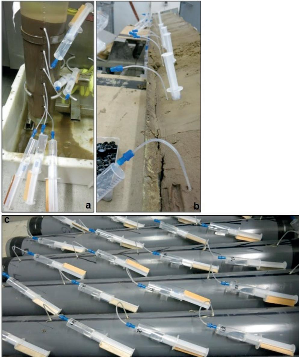
Fig. 10.9.1: Pore water sampling; a: Multi-corer tube (5 cm intervals); b: Box core sediment (20 cm intervals); c: Gravity corer segments (20 cm intervals)
