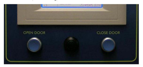
Pressing the EMERGENCY STOP button immediately stops any scanner or door movement and switches off the X-ray tube. To recover from an emergency stop pull the emergency stop button out and press the RESET EMERGENCY STOP button. To recover from an emergency stop also press the <u>RESET ERROR</u> and <u>RESET CYCLE</u> buttons at the touch screen. These buttons are available on the Main Menu screen.
