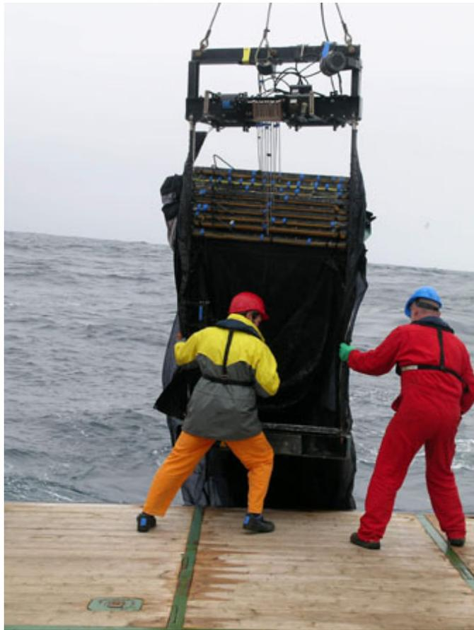
**Figure 3:** Deployment of the 1m<sup>2</sup>-MOCNESS with 9 netbags.
