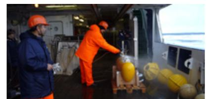
An instrument being rinsed after recovery. It harbors four years data of vertical temperature, salinity and velocity profiles. (Photo: I. Waddington)
