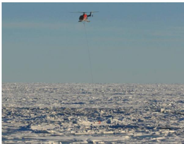
The EM Bird is carried on a 20 m long rope and flown at a height of ca. 15 m above the sea ice. (Photo: S. Hendricks)
