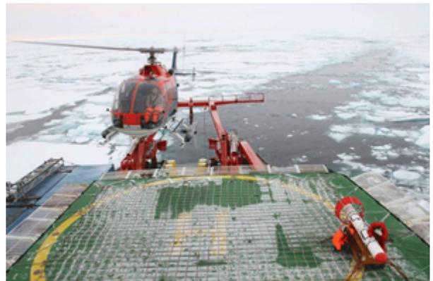
Take off of the helicopter for measurements of sea ice thickness with the EM-Bird (right). The operation requires an EM-Bird-operator and a person to observe the state of the sea ice. Priska and Robert (lower right) are getting the bird ready for its flight. (Photo: A. Ulfso)
