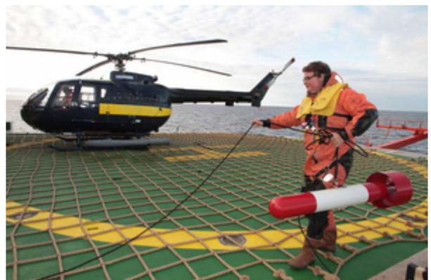
Preparing for an aeromagnetic survey flight; the sensor bird with the magnetometer in front. (photo: U. Stüwe)
