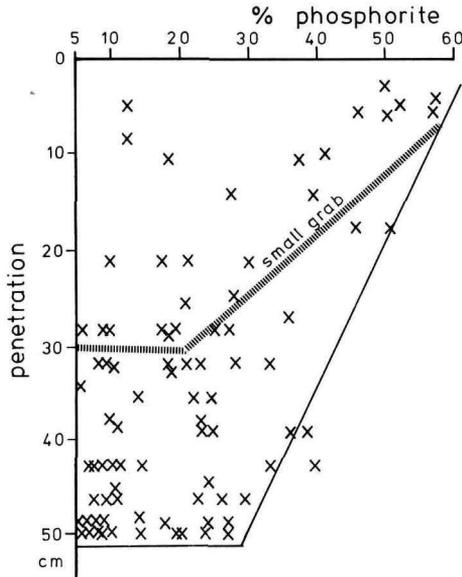
Fig. 4: Penetration of large pneumatic grab sampler versus phosphorite content. Only those SO-17-samples which did not reach the underlying chalk are plotted (x). Note the excellent penetration of the large grab in sediments with a phosphorite concentration up to 30 %, as compared to the small grab (used only during the VALDIVIA cruise), the values of which lie only above the dashed line.
