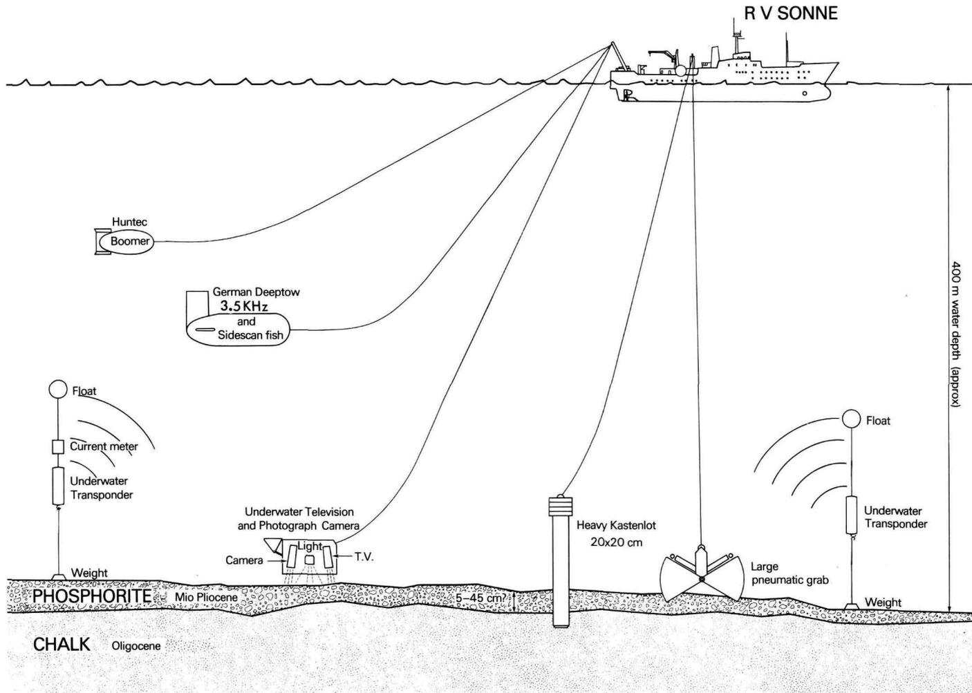
Fig. 2: Instrumentation, SO-17-cruise (scale of instruments not comparable).
