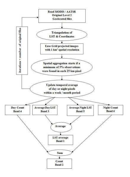
Figure 1: Processing flowchart for UW pan-arctic LST products
