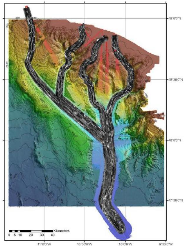
**Fig. 2:** JC35 (June 2009) EM120 multibeam and TOBI sidescan sonar coverage on the central Whittard canyon system (Huvenne, 2009).
