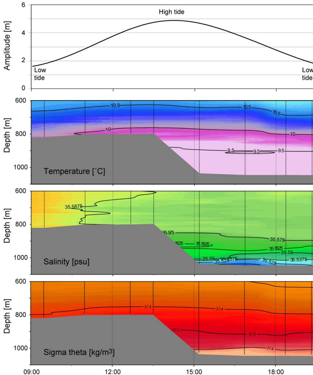
**Figure 9:** CTD casts collected with MUC between 09:00 a.m. and 19:30 p.m. (UTC) in relation to the tidal cycle from St. Mary's, Isles of Scilly, England. All presented parameters follow the tidal cycle at ~800 m water depth with an amplitude of ~50 m.
