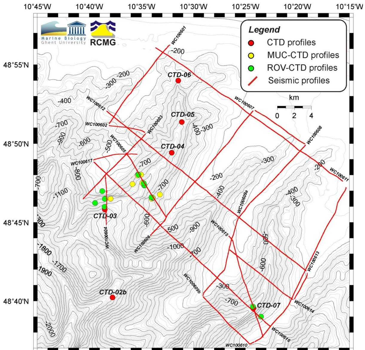
**Figure 3:** Location of seismic profiles (red line), CTD station (red circle), MUC stations (yellow circle) and the start/end of each ROV dive (green circle) within the middle branch of the Whittard Canyon system (INSS multibeam bathymetry).
