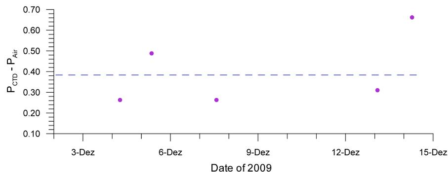
**Figure 2: Deviation of CTD pressure values from 0 dBar at sea surface.**
