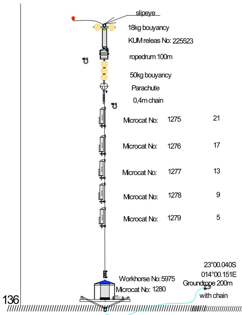
**Figure 3: Sketch of the mooring recovered during the cruise**
