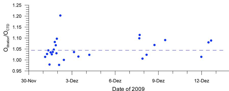
**Figure 1: Comparison between CTD oxygen concentration and Winkler titration of water samples.**
