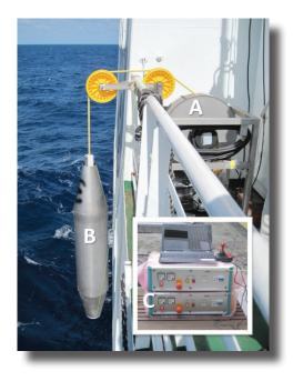
Fig. 3.8.2: Cable winch (A), underwater winch with casing (B) and deck units (C) of the new calibration system
