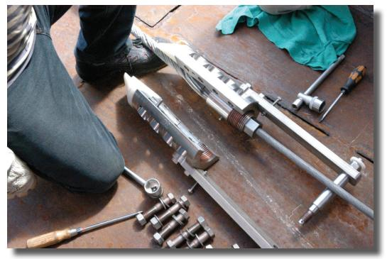
Fig. 3.9.2: The disassembled "AWI-GRIP®" termination
