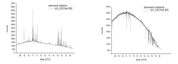
Fig. 3.1.2: Time series of downward radiance (left) and irradiance (right) for VIS at pixel 500 obtained from a measurement on Polarstern on 22 April 2011 (preliminary and uncorrected data).
