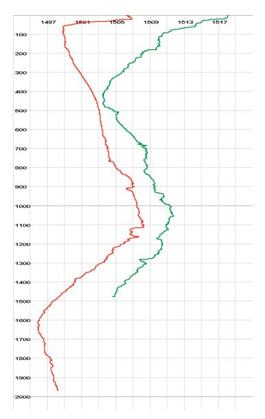
Fig. 3.5.1: Sound velocity profile of station PS77/329-1 (red) and PS77/332-1 (green). Vertical axis shows the water depth in meter, horizontal axis the sound velocity in meter per second.
