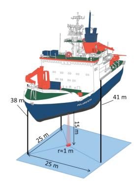
Fig. 3.8.1: Location of deployment of the three underwater winches or 'plumblines' (black vertical lines), respectively, and plain of calibration (blue area). Blue thin lines represent the lines connected to small calibration sphere. The red circle marks the sound beam area (radius ca. 1 m) in 15 m depth underneath the ship.
