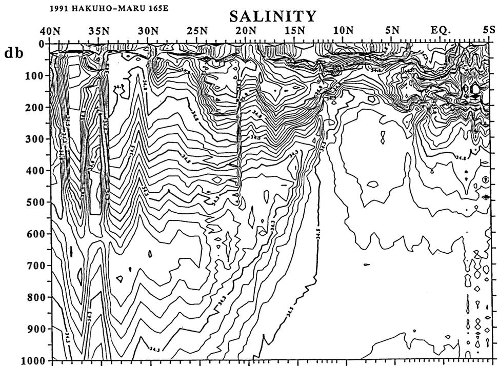
Figure 3 Vertical distribution of in-situ temperature (upper) and salinity (lower) at depths less than 1000 db along 165°E.
