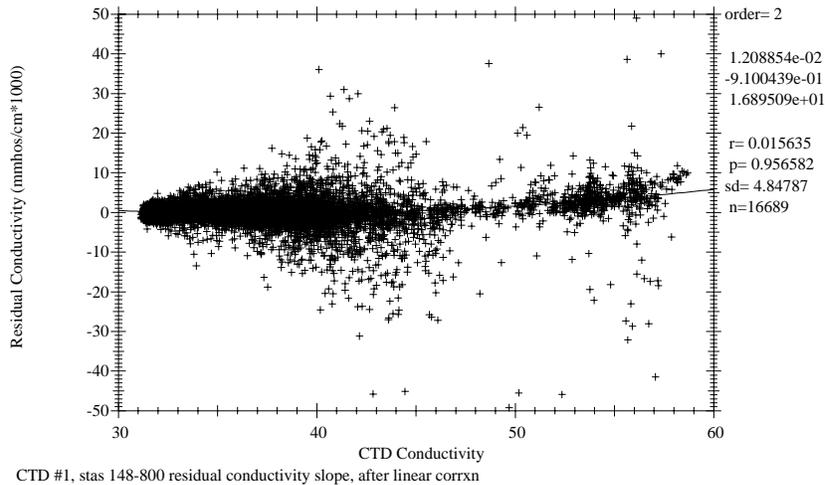
Figure 1.7.3.2 CTD #1 residual non-linear conductivity slope.
