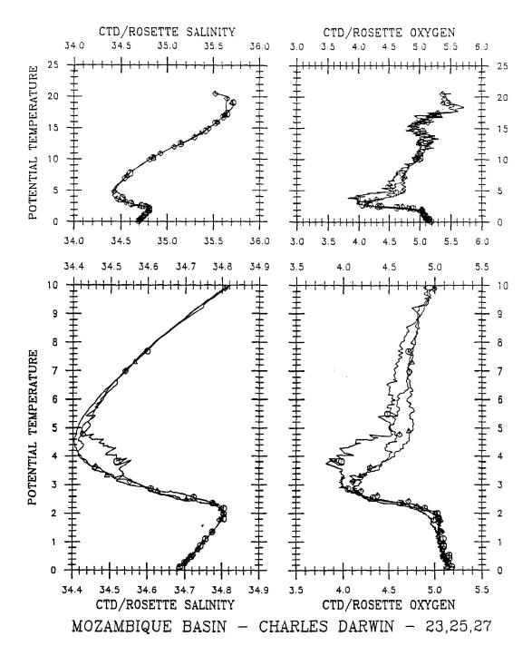
Fig.12 Typical potential temperature vs. salinity and oxygen plots from the Mozambique Basin during RRS Charles Darwin cruise #29. Symbols represent rosette water sample data for those particular casts. The bottom plots are expanded scale to show deep theta/property consistency.
