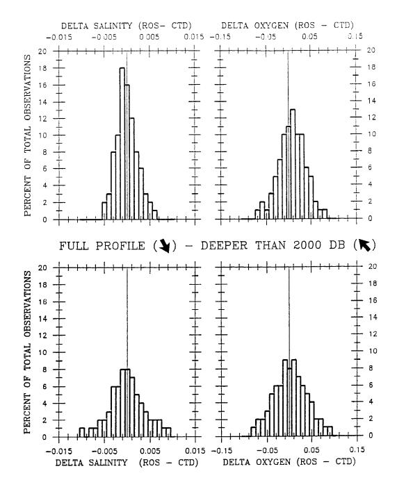
Fig. 7 Histograms showing the distribution of the salt and oxygen differences (CTD vs. rosette samples) for: Below: all stations at all depths. Above: all stations at depths greater than 2000 db.
