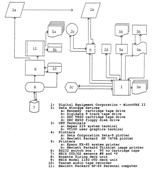
Fig. 2 Block diagrams of the CTD data collection and processing systems employed on the RRS Charles Darwin trans-Indian cruise.
