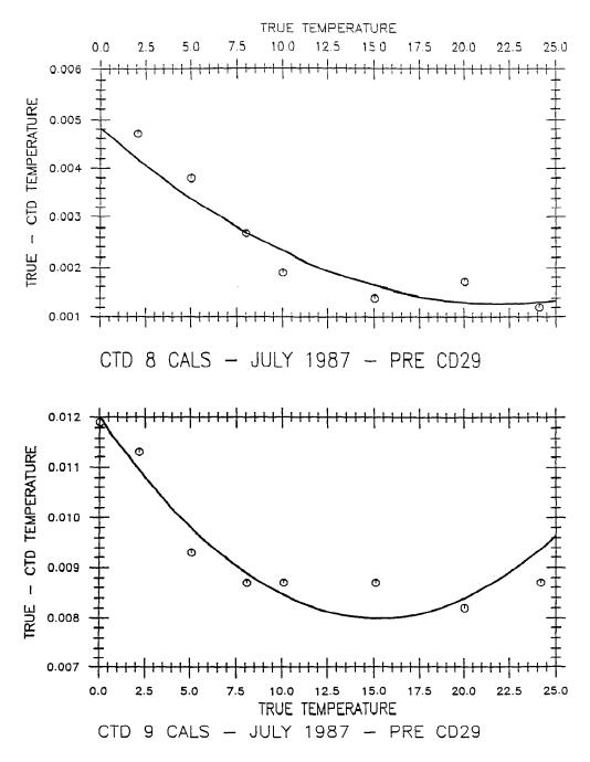
Fig. 3 Laboratory calibration data for the CTD temperature sensors along with quadratic least-square fits to the data used to reduce the CTD data.
