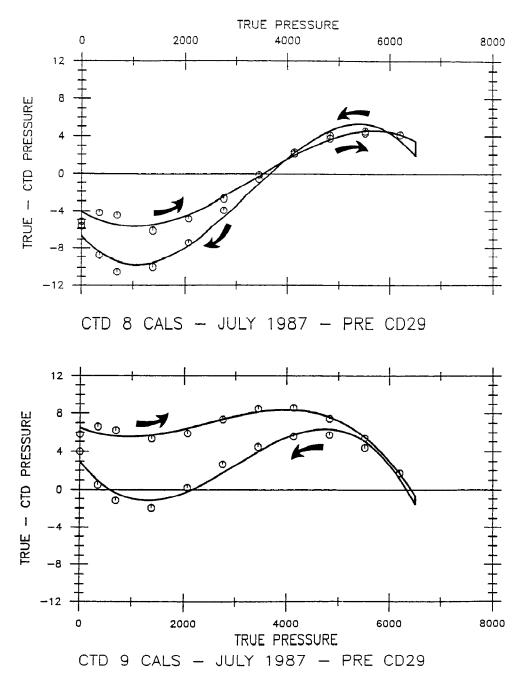
Fig. 4 Laboratory calibration data for the CTD pressure sensors along with cubic least-square fits to the data used to reduce the CTD data.
