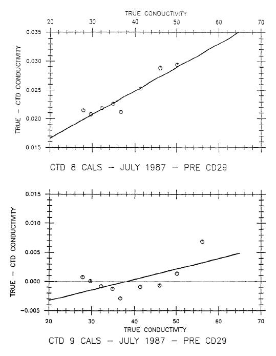
Fig. 5 Laboratory calibration data for the CTD conductivity sensors along with linear least-square fits to the data used to reduce the CTD data.
