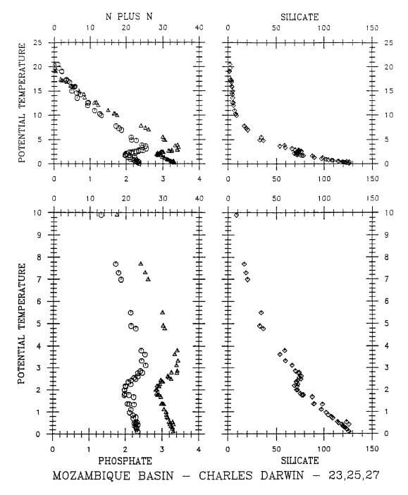
Fig.13 Typical potential temperature vs. nutrient data plots from the Mozambique Basin during RRS Charles Darwin cruise #29. Phosphate data are represented by triangles, N+N by circles, and silicate by diamonds. The ordinates (potential temperature axes) are at the same scales as Figure 12.
