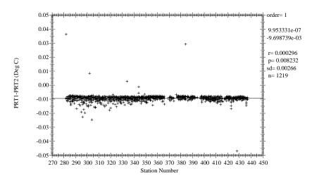
Figure 1.8.2.0 Shipboard comparison of CTD #1 primary/secondary PRT temperatures, pressure > 1800 db.
