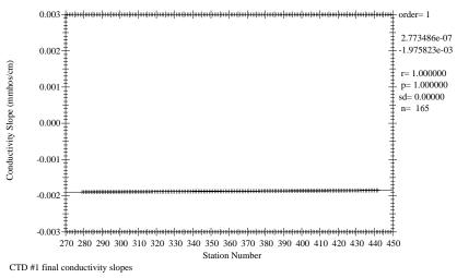
Figure 1.8.3.3 CTD #1 conductivity slope corrections by station number.
