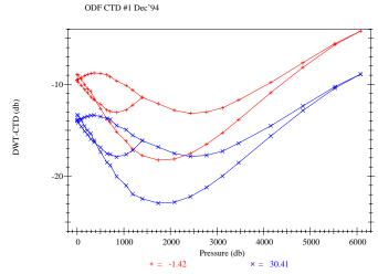
Figure 1.7.0 Pressure calibration for ODF CTD #1, December 1994.
