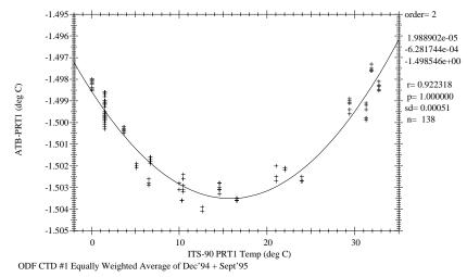
Figure 1.8.2.1 Primary temperature correction for ODF CTD #1, Dec.94/Sept.95 equally weighted average.
