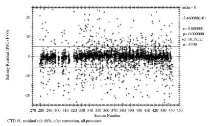
Figure 1.8.3.6 Salinity residual differences vs station # (after correction).
