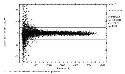
Figure 1.8.3.5 Salinity residual differences vs pressure (after correction).
