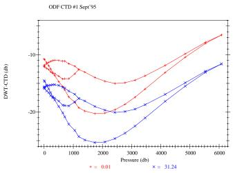
Figure 1.7.1 Pressure calibration for ODF CTD #1, September 1995.
