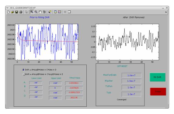
Figure 43 Example IES\_GUIDEDRIFT2EXP window showing expanded view of data prior to fitting drift (left) and after drift removed (right)
