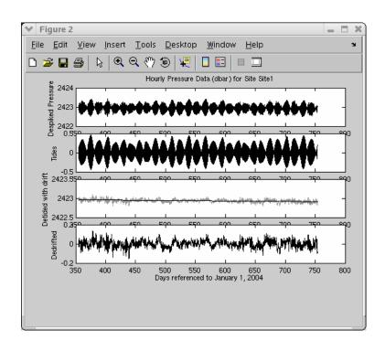
Figure 66 Example Figure 2 window showing the despiked pressure, tides, detided pressure with drift and dedrifted pressure time series
