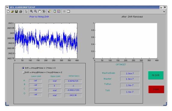
Figure 41 Example IES\_GUIDEDRIFT2EXP window prior to fitting drift
