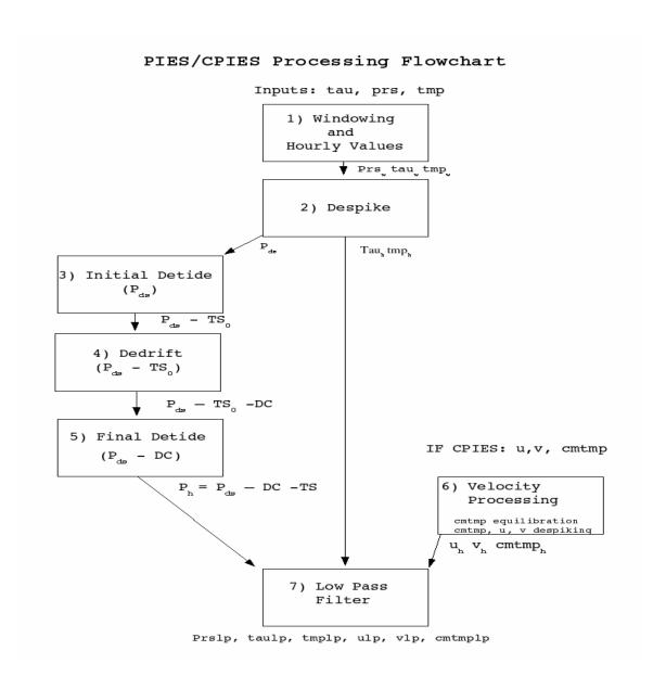
**Figure 4 IES Data Processing Flowchart**
