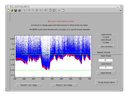
Figure 20 Example IES GUITAULIMITS window with reduced Y-axis range
