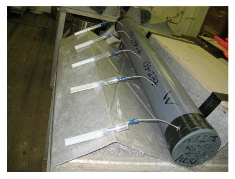
Fig. 42: Segments of Gravity Core sampled with rhizons and plastic syringes
