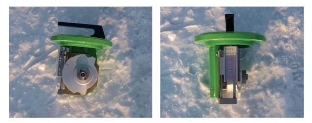
Fig. 66: 24 Hours Assembly with coated Sampling Slide
