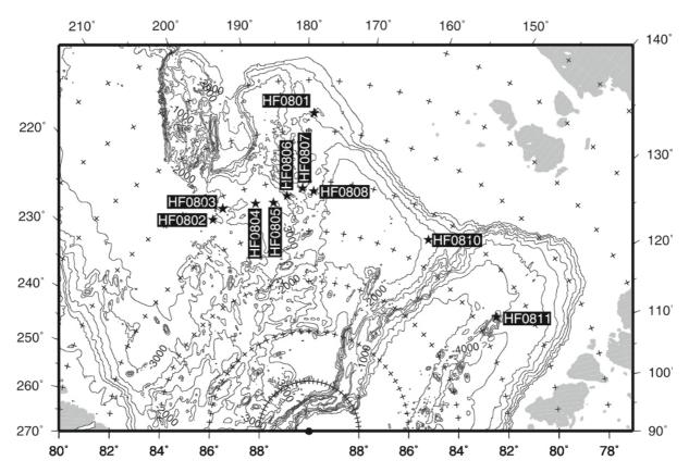
Fig. 50: Bathymetric map of the study area during ARK-XXIII/3 with observed heatflow values [mW/m<sup>2</sup>]. Contour interval is 500 m.
