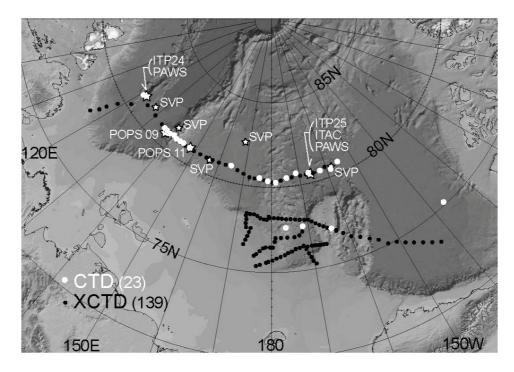
Fig. 52: Seafloor bathymetry with locations of CTD casts (white dots) and XCTD casts (black dots) and buoy deployments (labels)
