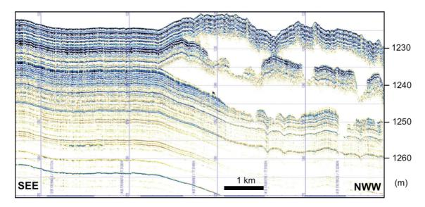
Fig. 9: Parasound example from the Arlis Plateau. Coring location PS72/343 is on left end of the profile. Data processing: negative flank suppressed
