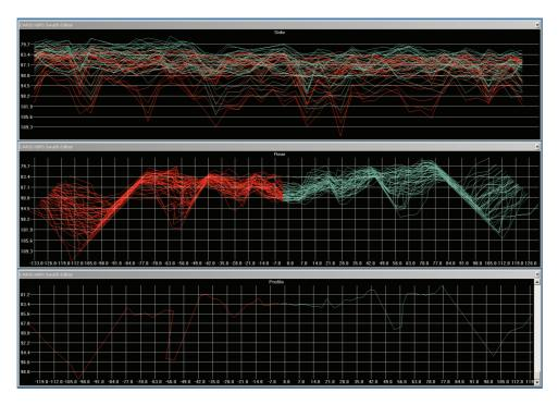
Fig. 62: Wrong depth measurements in shallow water
