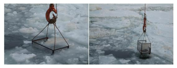
Fig. 47: Collecting pieces of drift ice by using the ship's crane
