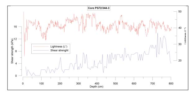
Fig. 14: Shear strength of core PS72/344-3 from the Arctic Ocean plotted together with the lightness record of the same core. The gradual increase in shear strength is typical for normal consolidation processes.
