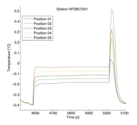
Fig. 51: Extraction from the recorded temperature data at station HF0807A01 (PS72/413). Position numbers indicate the logger's depth below seafloor (01, 5.86 m; 02, 6.69 m; 03, 7.63 m; 04, 8.60 m; 05, 9.54 m). Penetration of the gravity corer into the sediment is followed by an increase in temperature. While pulling the device out of the sediment after five minutes a friction heat pulse occurs.
