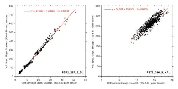
Fig. 12: Correlation of MS data measured with a loop sensor and converted to volume-specific MS with MS data measured with a point sensor.
