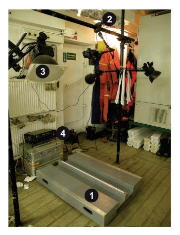
Fig. 21: On-board photography system. Numbers label the different parts where particular attention is required. 1 the support orientation. 2 the room light intensity. 3 spot orientation. 4 spot light intensity control. 286
