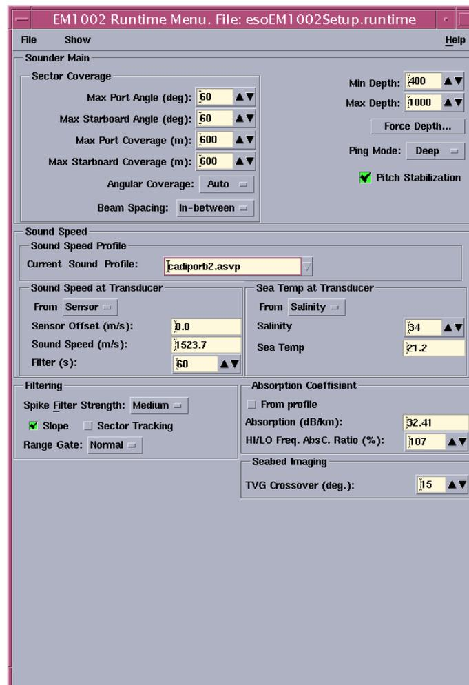
**Figure 13:** Screenshot of the multibeam input parameters concerning sound velocity and filtering.
