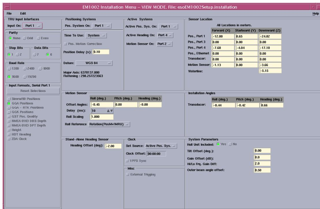
Figure 12: Screenshot of the multibeam input parameters concerning motion sensors and roll/pitch calibration.
