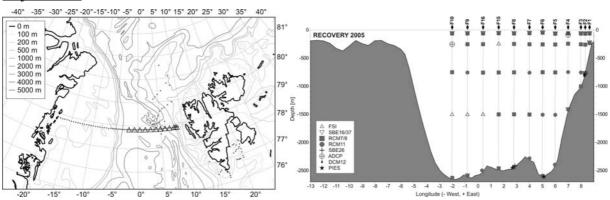
Fig. 3.1: Location of CTD stations and moorings (left) and distribution of instruments at the mooring array (right) recovered and redeployed in 2004.
