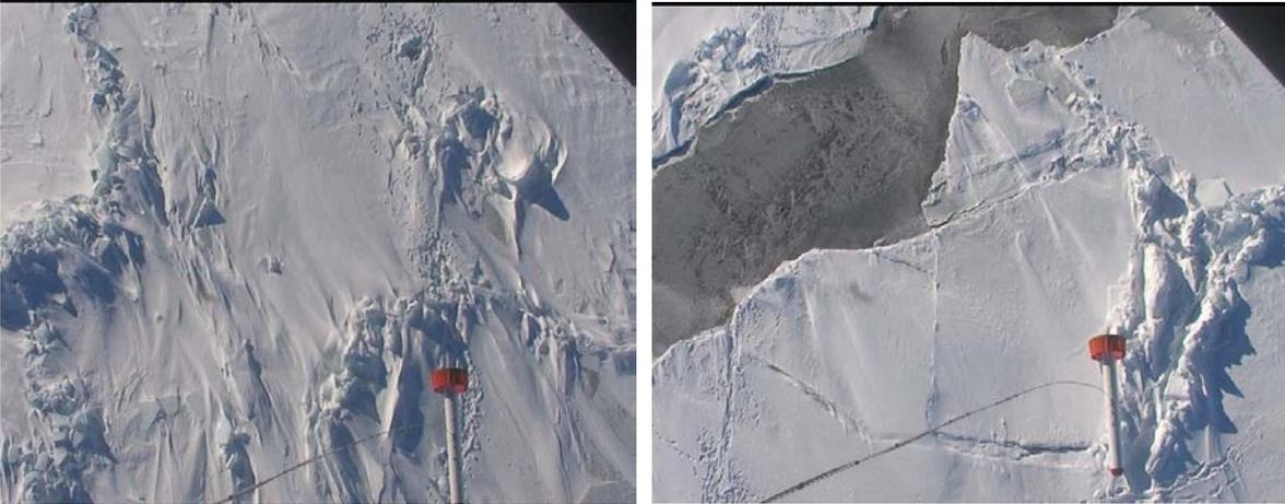
**Figure 15:** Photographs obtained from nadir video camera showing varying agreement between HEM flight track and ground profile (visible by footsteps in the snow).
