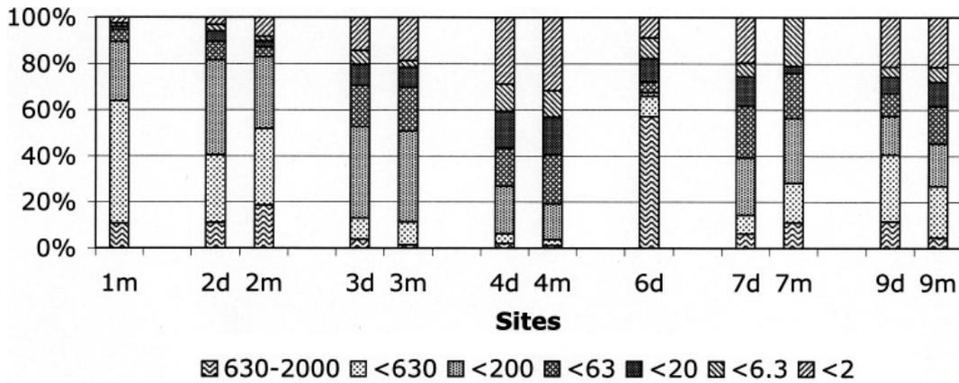
**Fig. 2:** Shares (wt.%) of grain sizes ( $\mu\text{m}$ ) of soil samples (Leg 1, TNW-99).
