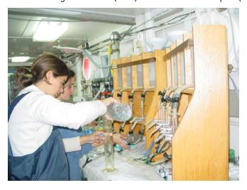
Fig. 6 Filtration of Seawater on board for Particulate Organic Carbon (POC) and Lipid analysis.
