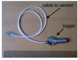
**Figure 9.** The in resin embedded Inter-Mandibular Angle Sensor (IMASEN) used on the harbour seals, showing the cable linking the Hall sensor to the logging unit.
