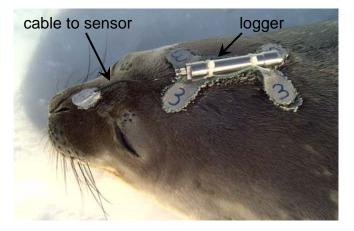
**Figure 10.** The titanium-housed Inter-Mandibular Angle Sensor (IMASEN) deployed on a Weddell seal.
