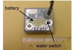
**Figure 7.** The satellite transmitter (PTT) SPOT2-tag from Wildlife Computers.
