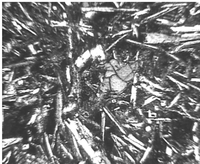
*Fig.7.41: Euhedral olivine phenocryst surrounded by glass-plagioclase microlite matrix*
