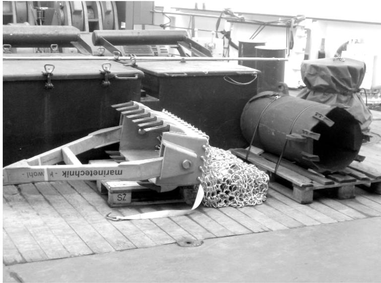
Fig. 7.4: Frame and barrel dredges used on ARK-XX/2
