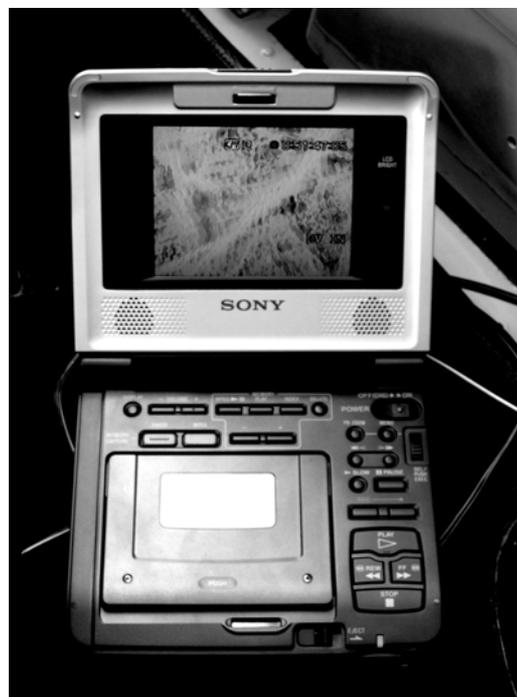
*Fig. 4.5.1.3: Video recorder with display in the interior of the helicopter. From here the video recording could be started and stopped and with the display the correct functionality of the camera was monitored.*
