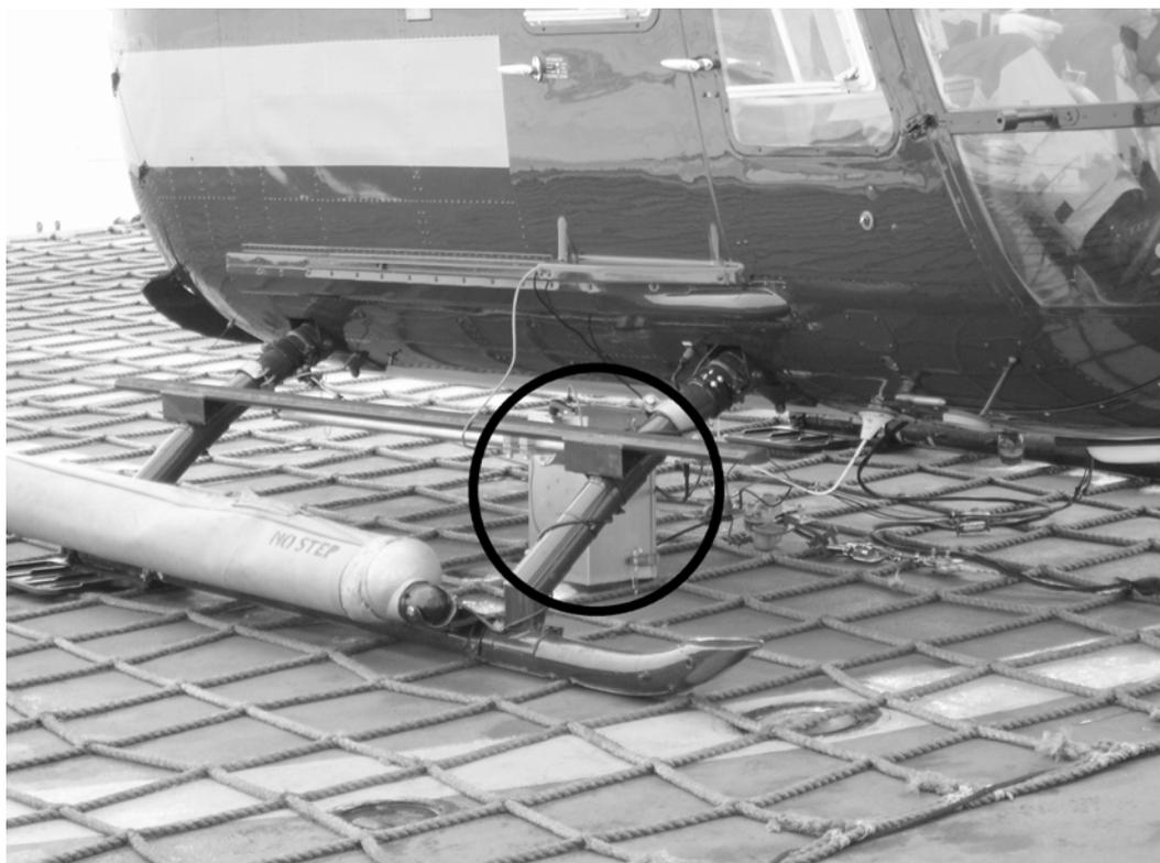
*Fig. 4.5.1.2: Video camera in a metal box mounted below the helicopter. The cables to the interior of the helicopter used for the temperature stabilization of the box and for the video stream to the video recorder are visible, too.*
