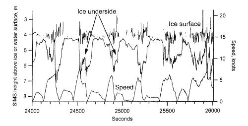
Fig. 24: Half-hour section of SIMS profile from September 14, showing laser and EM-data as well as ship's speed.
