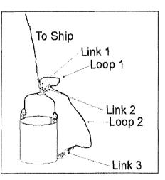
Figure 61: Rigged dredge.
