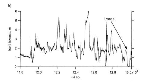
Fig. 26a+b: Typical section of a HEM profile, showing a) the height above the ice or water surface as determined by means of laser altimetry and EM induction, and b) the resulting ice thickness.
