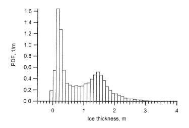
Fig. 25: Typical thickness distribution derived with the Sea Ice Monitoring System. PDF = Probability Density Function.
