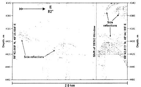
Fig. 46 An example of a poor acoustic PARASOUND record affected by side reflections. Central part of the rift valley.
