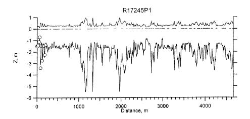
Fig. 20: The longest ground-based thickness profile ever surveyed on an Arctic ice floe. Surface elevation and draft are shown. These were calculated from ice thickness assuming an ice density of 880 kg/m<sup>3</sup>. The ticks and lines at Z = 0 m demarcate the location of melt ponds. See Fig.19 for Z.
