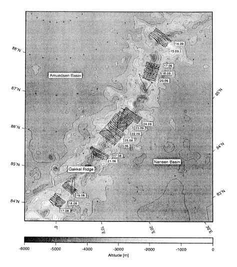
Figure 84: HELIMAG profiles along the Gakkel Ridge. The grey shade and contour lines (500 m interval) show bathymetric depths taken from IBCAO data. Black lines mark the flight paths. Dates of flights are indicated.
