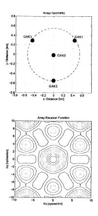
Figure 90: The arrangement of the seismological array and its receiver characteristics.
