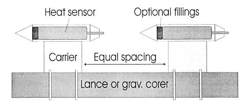
Figure 86: Heat flow set-up.
