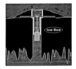
Figure 95: Sketch of the deployment of a MT-sensor.
