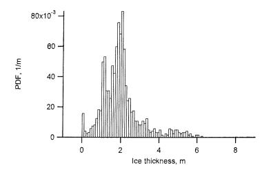
Fig. 27: Thickness distribution for the profile in Fig. 26.
