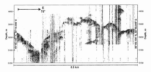
Fig. 51. PARASOUND record from sediment-lacking rift valley of the central segment of the Gakkel Ridge (PARADIGMA online printout). Note presence of the side echoes and very rough topography of the floor, which is considered as a result of recent volcanic activity.
