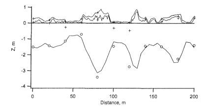
Fig. 19: Typical example for a baseline profile (Station 245). The elevation of the snow and ice surface obtained from surveying is shown, as well as the electromagnetically derived ice draft (lines). The crosses and circles indicate the respective data from drill-hole measurements. Snow-covered melt-ponds are present at 50, 100, 145, 155, and 190 m.
