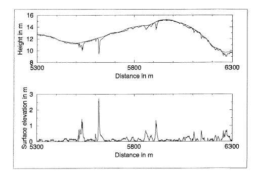
Figure 29: One-kilometer section of a laser profile. The raw data and the helicopter motion derived from it are shown (top) as well as the resulting profile of surface height (bottom).
