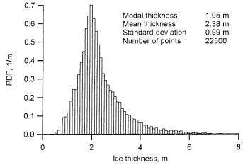
Fig. 23: Thickness distribution of all ground-based EM measurements. PDF = Probability-Density-Function.
