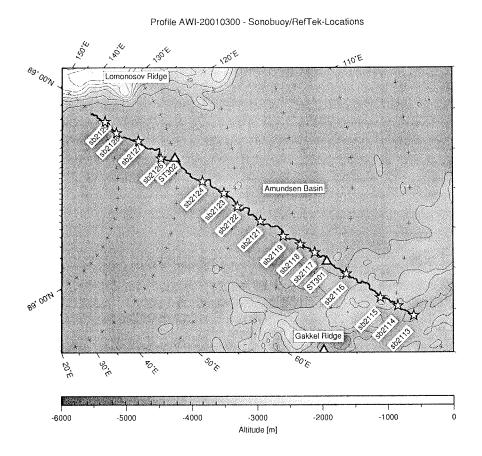
Fig. 79: Location map of the seismic profile in the Amundsen Basin. The stars indicate the positions were sonobuoys were dropped.
