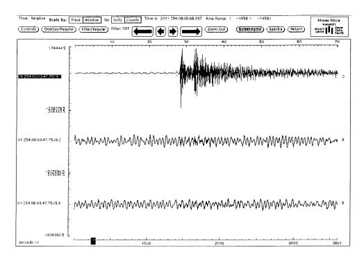
Figure 91: Record of a local earthquake at a single station (GAK21) of array GAK-2: Trace 1 above displays the vertical component, Trace 2 in the middle the horizontal components in NS-direction and trace 3 at the bottom the horizontal component in EW direction of the seismometer. Note the typically high amplitudes on the vertical component compared to the low amplitudes on the horizontal components.
