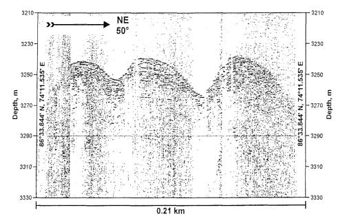
Fig. 45 An example of the PARASOUND DESO record with periodically repeated reflection pattern due to ice ramming above the same sea-bottom feature. Although the time interval recorded is about 20 min, the distance of the total ship movement is 0.21 km only.
