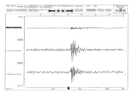
Figure 92: Typical record of an ice-quake at a single station (GAK-21) of array GAK-2. Trace 1 above displays the vertical component, Trace 2 in the middle the horizontal components in NS-direction and Trace 3 at the bottom the horizontal component in EW direction of the seismometer. Note the characteristically high ratio of amplitudes of the horizontal components compared to the amplitudes of the vertical component.
