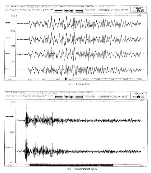
Fig. 93: Teleseismic events: a) Hokkaido earthquake: vertical components of stations at detection array GAK-0; b) Greenland Sea: vertical components at the refraction station 201; Note the different frequency contents of the two quakes compared to the same timescale (100s).
