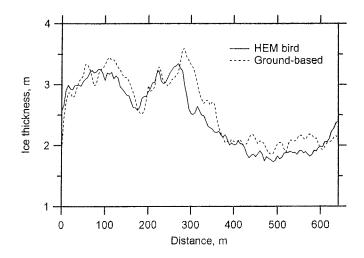
Fig. 28: Comparison of HEM and ground-based thickness profile.
