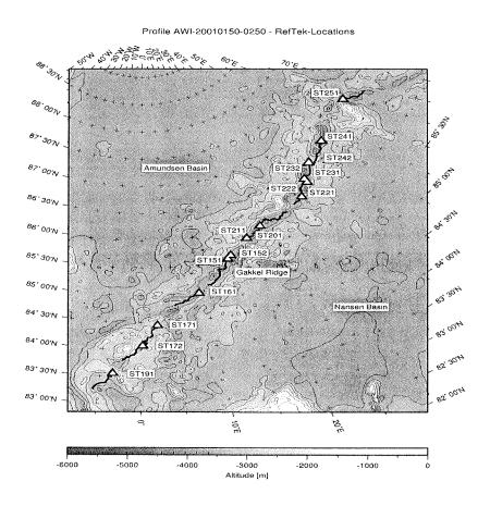
Figure 82: Location map of the seismic refraction profiles along Gakkel Ridge. The stars indicate the positions of the RefTek recording instruments along each profile.
