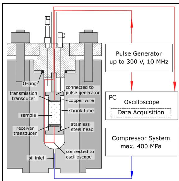
645 **Figure 3.** Schematic of the experimental setup used to determine the P-wave velocities under confining pressure. This setup comprises a pressure vessel with a sample chamber, pulse generator, compressor control, and PC-based acquisition unit. Placed inside the oil-filled pressure chamber there is the sample assembly (Barblan, 1990).
