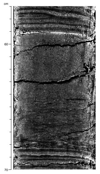
Figure 10. Photograph of a thin massive interval within laminated sediment showing discontinuous/disrupted laminae at the base, grading to entirely homogenous mud. A characteristic pale diatom ooze lamina marks the top (interval 169S-1033B-4H-4, 56–70 cm).
