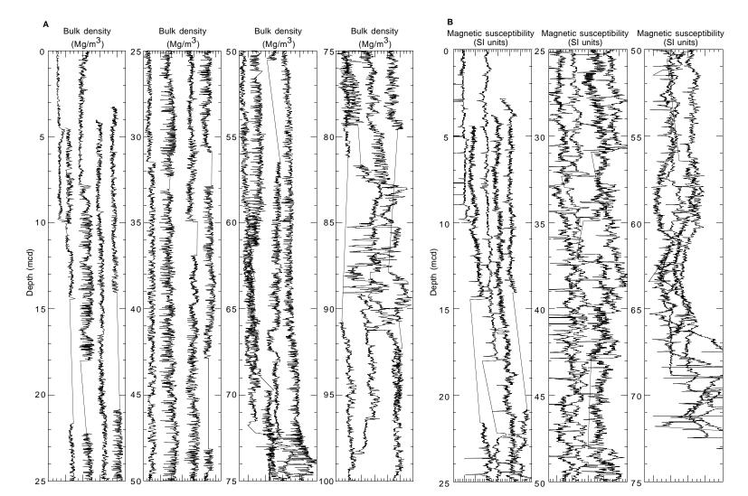
Figure 23. **A.** GRAPE bulk density data vs. depth for all holes at Site 1034. The density scale has ranges of  $1.6 \text{ Mg/m}^3$  for 0-25 mcd,  $1.4 \text{ Mg/m}^3$  for 25-50 mcd,  $1.9 \text{ Mg/m}^3$  for 50-75 mcd, and  $1.2 \text{ Mg/m}^3$  for 75-100 m. **B.** Magnetic susceptibility vs. depth for all holes at Site 1034. The scale has ranges of 75 SI units for 0-25 mcd and 50-75 mcd, and 70 SI units for 25-50 mcd. (continued on next page).
