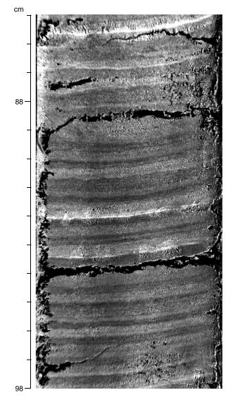
Figure 6. Photograph showing characteristic laminated muds of Unit I. The paler laminae are diatom ooze; the darker laminae are diatomaceous mud and the occasional very light sub-laminae are silty muds (interval 169S-1034B-3H-6, 85–98 cm).
