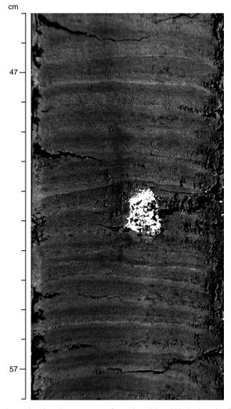
Figure 14. Pale yellow aggregate of granular calcite within laminated sediment in interval 169S-1034B-5H-2, 45–58 cm. This is thought to result from the decomposition of a calcium carbonate hexahydrate crystal (ikaite).
