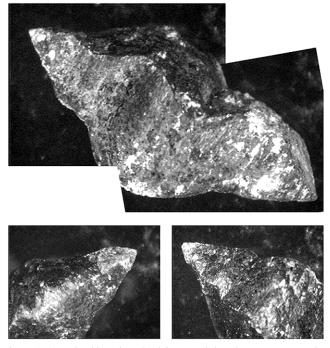
Figure 15. Angular, biterminated calcite crystal thought to represent a glendonite pseudomorph of calcium carbonate hexahydrate (ikaite; Sample 169S-1034D-7H-1, 76 cm).
