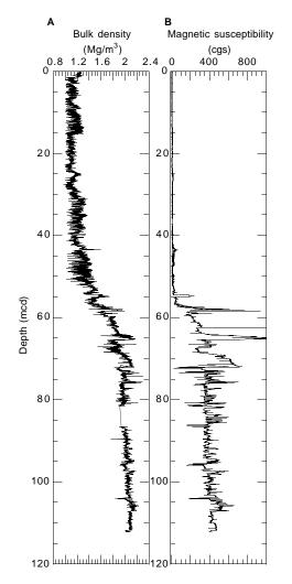
Figure 21. A. Composite of the spliced bulk density record vs. depth for Site 1033. B. Composite of the spliced magnetic susceptibility record vs. depth for Site 1033.
