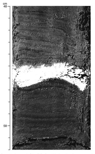
Figure 11. Photograph of the distinctive ash horizon thought to represent the Mazama Ash (interval 169S-1033B-5H-6, 48–60 cm).
