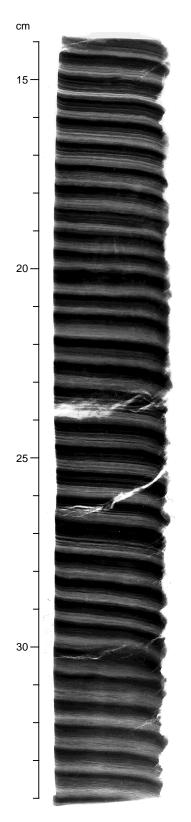
Figure 16. Print of X-ray radiograph of laminated sediments from interval 169S-1034B-4H-3, 14–34 cm. The centimeter-scale pale (diatom-rich) dark (terrigenous sediment-rich) alternations represent annual "varves." Within these annual varves, up to 10 intra-annual sub-laminae are present.
