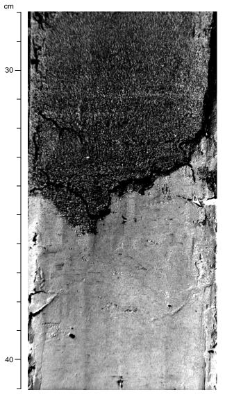
Figure 13. The irregular erosive base to a sand layer in Unit II (interval 169S-1033B-7H-2, 27–41 cm).
