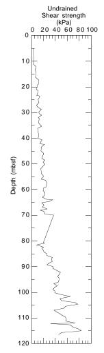
Figure 25. Undrained shear strength vs. depth for Hole 1034B.
