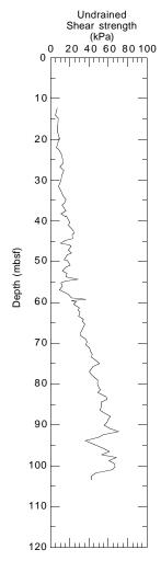
Figure 22. Undrained shear strength vs. depth for Hole 1033B.
