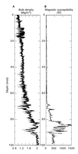
Figure 24. **A.** Composite of the spliced bulk density record vs. depth for site 1034. **B.** Composite of the spliced magnetic susceptibility record vs. depth for Site 1034.
