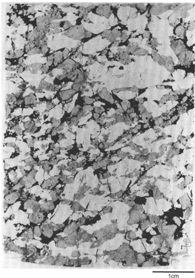
Figure 20. Plane light photograph of thin section showing slightly deformed iron-titanium oxide gabbro (118-735B-52R-4, 88-94 cm, Piece 4B). Elongated plagioclase (white) and pyroxene (gray) crystals define a primary igneous lamination cut by several microfaults. Redistribution of opaque minerals (black) along these microfaults clearly defines a foliation due to deformation.
