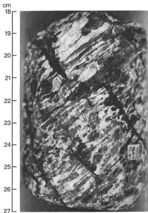
Figure 11. Amphibole veins perpendicular to the foliation in a well-foliated to augen gneissic gabbro (118-735B-85R-4, 18–27, Piece 1C).
