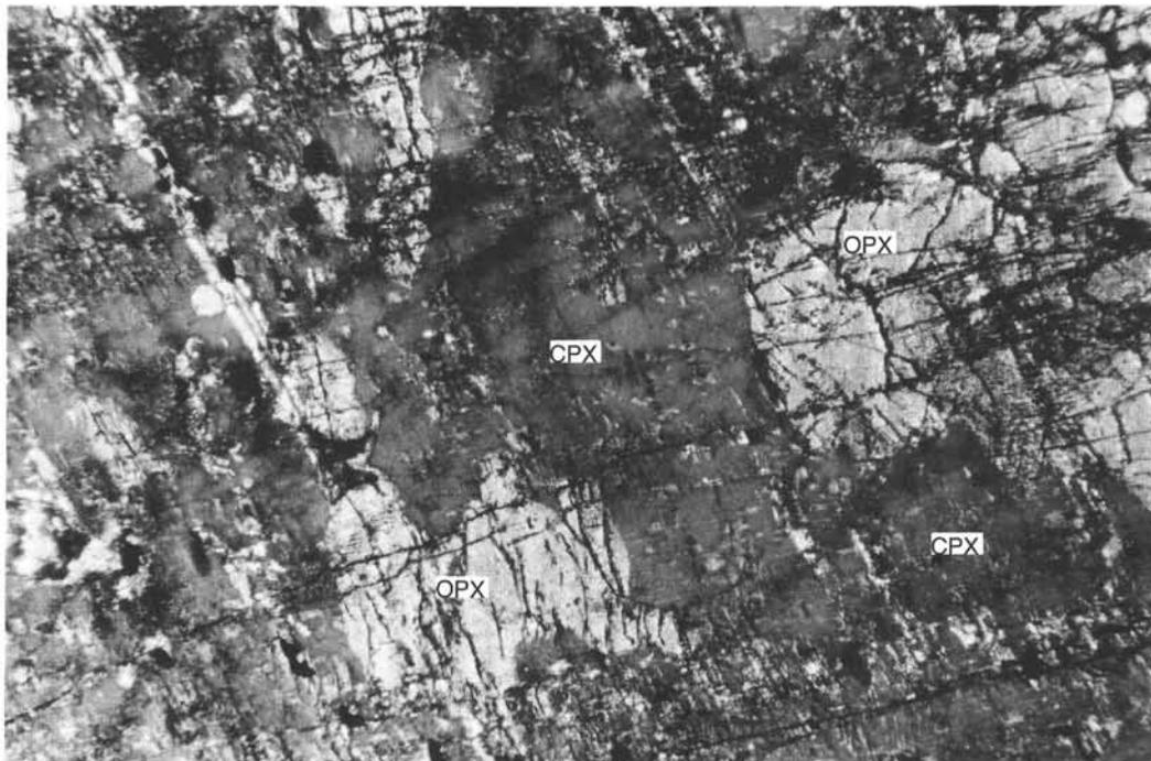
Figure 22. Polarized light photomicrograph of patchy orthopyroxene (OPX) in clinopyroxene (CPX). Field of view is 2.5 mm (118-735B-34R-4, 8–12 cm, Piece 2).
