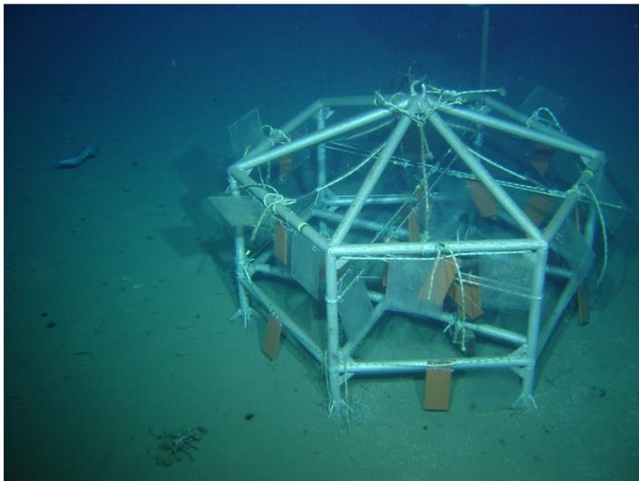
*Fig. 2.6: Metal frame with different kinds of hard substrates deployed in 1999 at the central HAUSGARTEN site HG-IV*
