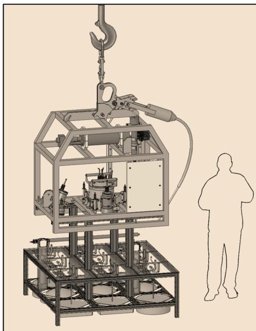
Fig. 2.4: Schematic view of the one-way deployment module (bottom) attached to a launcher system (top)
