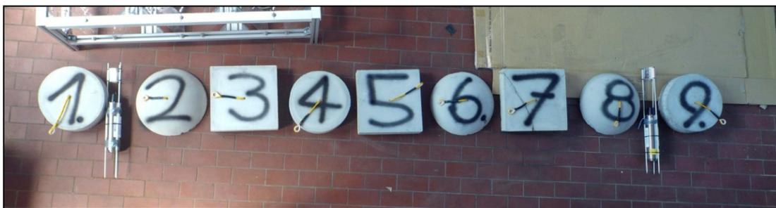
Fig. 2.3: Artificial dropstones and cylindrical homer beacons for tracking the stones at the deep seafloor laid out in a workshop before shipment
