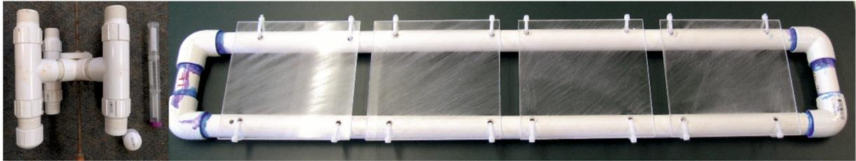
*Fig. 2.5. Embedded funnel larval trap design (left side) and settlement plates (right side)*
