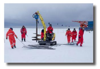
Fig. 3.1.1.7: The earthmover drives on plates to the drill site. The plates are necessary if the ice floes are covered with high and soft snow.
