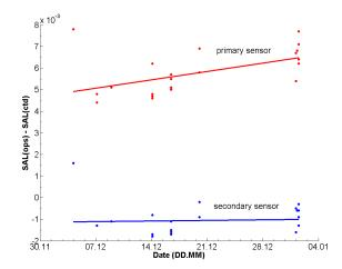
Fig. 3.1.1.5: Deviation in salinity between OPS measurements and in-situ CTD measurements for samples below 4,000 m depth. The correction for the secondary sensor (blue line) is about -0.0011, and constant over time, contrasting a notable drift of the primary sensor.
