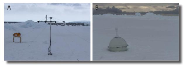
Fig. 3.2.1.5.1: a) Snow depth buoy combined with an IMB (yellow Pelicase), b) SVP buoy
