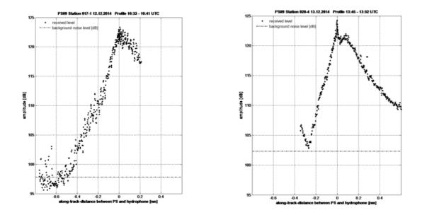
Fig. 3.1.6.2: Received broad band sound pressure levels ( $dB_{SPL}$  re 1µPa) as a function of Polarstern's distance from the CPA(closest point of the approach). Values less than zero represent the approach towards, values greater zero the departure from the CPA.
