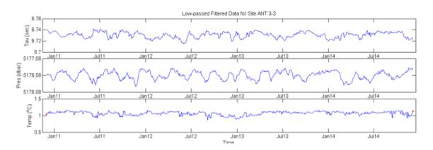
*Fig. 3.1.5.3: ANT 3-3 travel time, pressure and temperature data after processing. The red dots at the start and end of the temperature time series indicate the CTD's bottom temperatures.*
