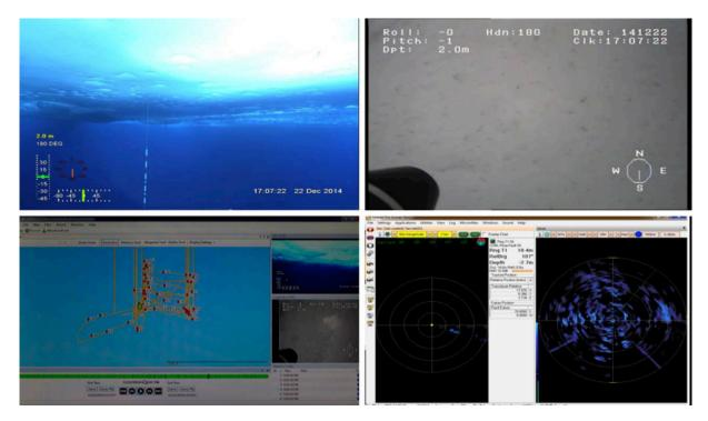
Fig. 3.2.1.4.3: Overview of the four operation screens. Upper left: Front camera. Upper right: Upwardlooking camera. Lower left: Positioning system based on USBL. Lower right: Sonar signal and distance between ROV and sea ice (top right corner)
