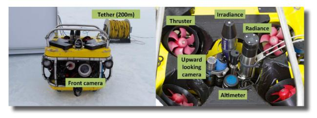
Fig. 3.2.1.4.1: Photograph of the ROV (left) and a close-up of the sensor side on top. The tether in the background contains the power line and allows for the communication between the vehicle and the ROV control hut (see Fig. 3.2.1.4.2).
