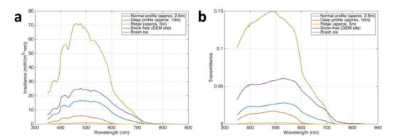
*Fig.* 3.2.1.4.6: Preliminary results (spectra) of station PS89/035-1 (22.12.2014). (a) Spectral irradiance under sea ice. (b) Spectral transmittance of snow and sea ice. In both figures spectra beneath different surface characteristics (or/and different depths) are shown: Level ice (diving depth: 2.5 m, blue), level ice (diving depth: 10 m, orange), old pressure ridge (diving depth: 5 m, yellow), snow free sea ice (diving depth: 2.5 m, purple), brash ice (2.5 m, green).
