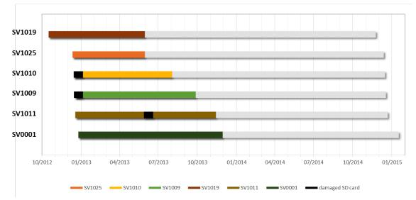
Fig. 3.1.4.2: Overview of deployment and operational period of acoustic recorders recovered during PS89. Grey bars indicate the deployment periods, while colored bars are indicative for actual recording periods of the recorders. Black bars represent periods during which recorders presumably operated but collected data have not yet been retrieved or backed up due to damaged SD cards.
