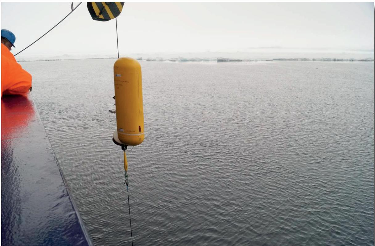
*Fig. 8.3: Deployment MMP- profiler*
