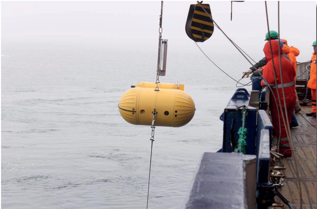
*Fig. 8.2: Subsurface winch and profiler during deployment*
