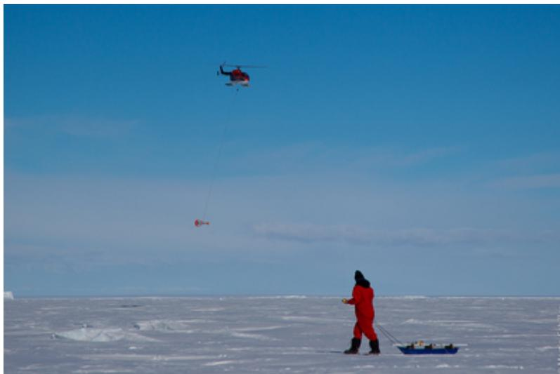
Fig. 3: The helicopter towed EM bird passes the GEM. © Martin Schiller, AWI
