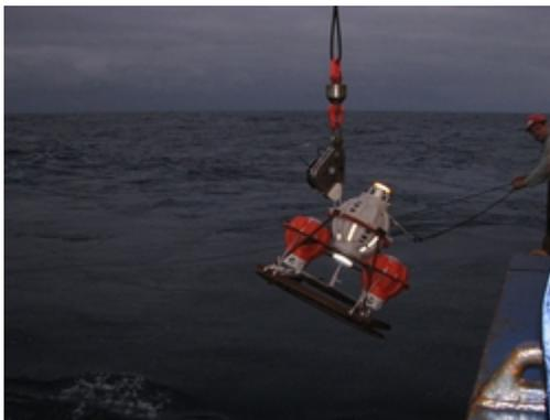
Fig. 1: Night-time deployment of a PIES (Pressure sensor equipped Inverted Echosounder). © AWI
