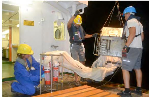
*Deployment of the multi net at night (photo D. Nürnberg).*
