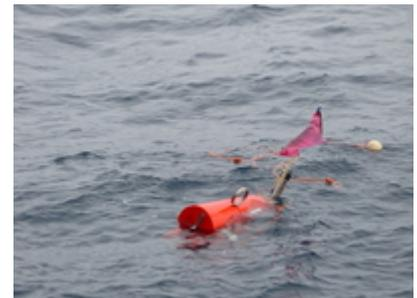
Fig. 2: Surfaced OBS. Note close to the flag the radio transmitter (Novatech) and beacon
