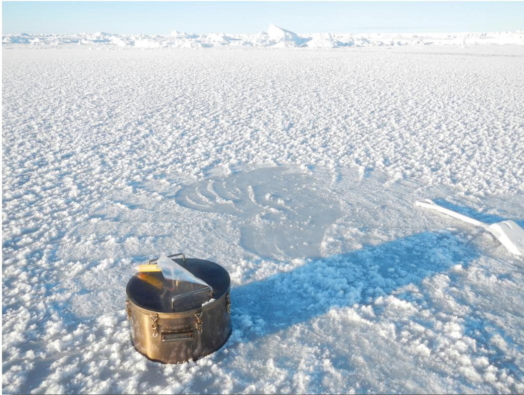
Fig. 6.4: Picture showing the metal chamber for VOC flux measurements over the frost flower at St. 517, 31 July 2013
