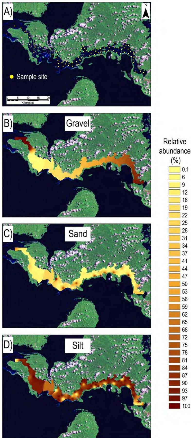
Figure 101 Sediment sampling program showing A) sites sampled and interpolated B) gravel, C) sand and D) silt fractions.
