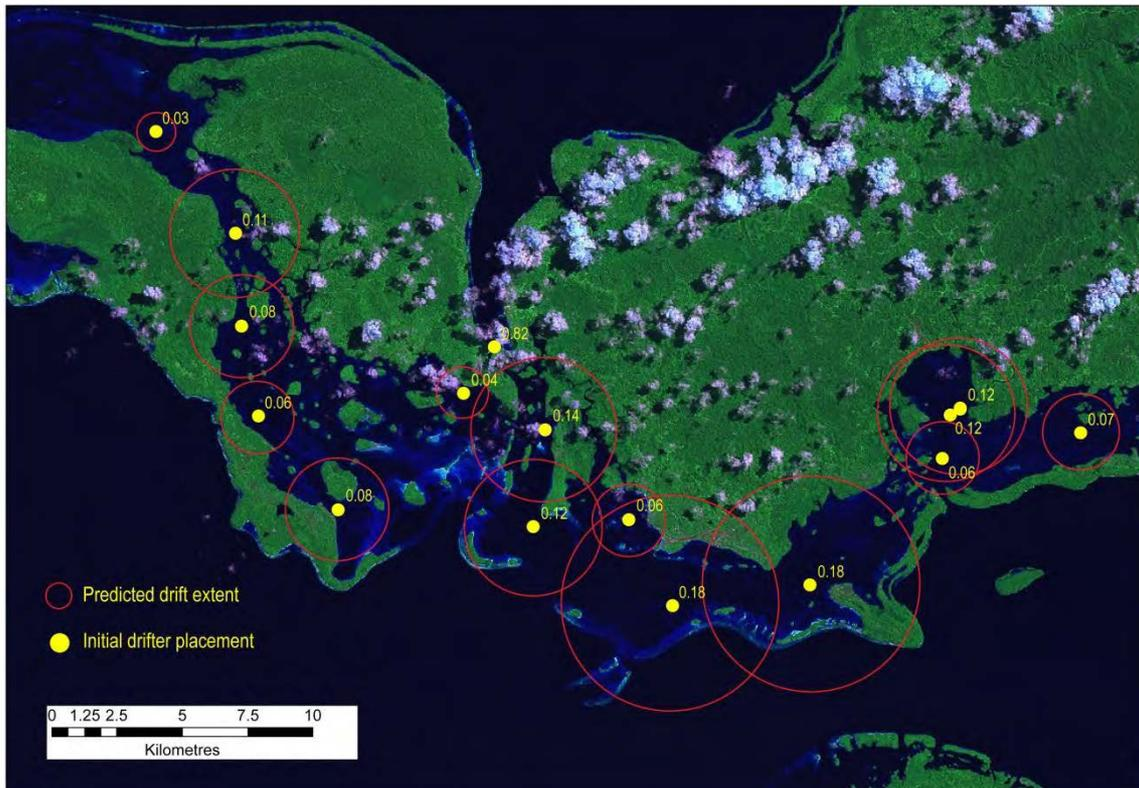
**Figure 107** Initial drifter deployment site and average drift rate during ebbing tide. Units  $m s^{-1}$ . Indication of predicted drift extent based on drifter track, note central site of Noro Passage has no drift extent as this is beyond the boundary of the figure.
