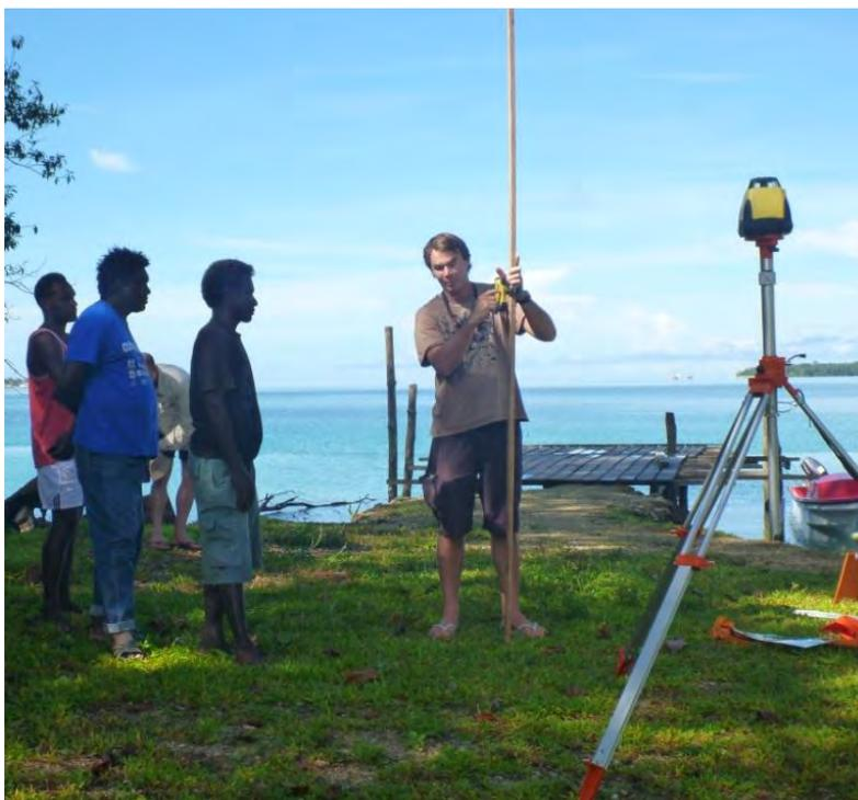
**Figure 36 Training RCF zone co-ordinators in the use of laser level survey equipment**
