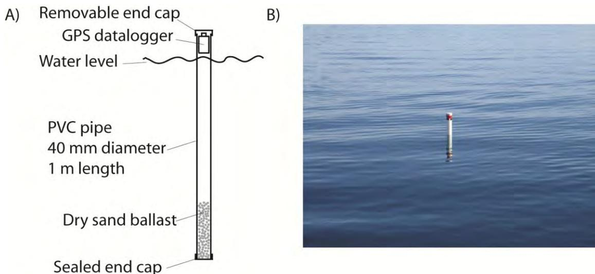
**Figure 105 A) Design of drifter used to monitor water currents and B) profile of drifter during deployment.**
