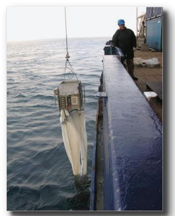
*Fig. 4.1: Deployment of the Multi net to collect mesozooplankton in the HAUSGARTEN area*
