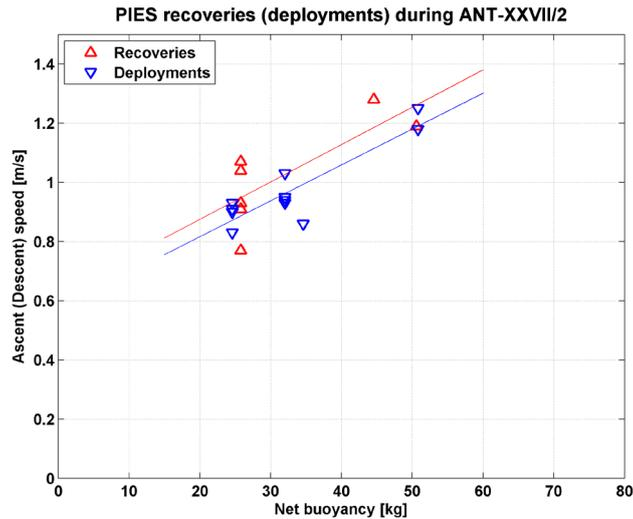
Fig. 2: Observed ascent and descent speed during PIES recoveries (red  $\nabla$  and deployments (blue  $\nabla$ ) as a function of net buoyancy. Note that for better comparison, both recoveries and deployments have been plotted with the absolute values of speed and net buoyancy.
