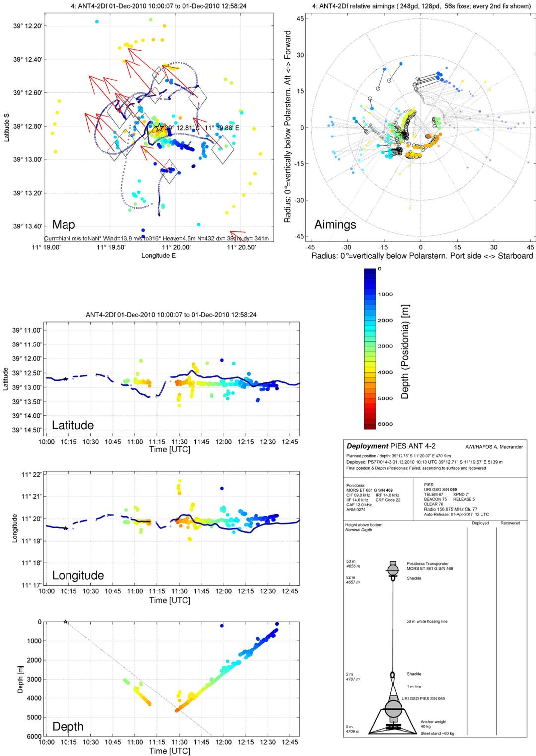
PIES deployment failed, as PIES release broke when the mooring hit the bottom.
