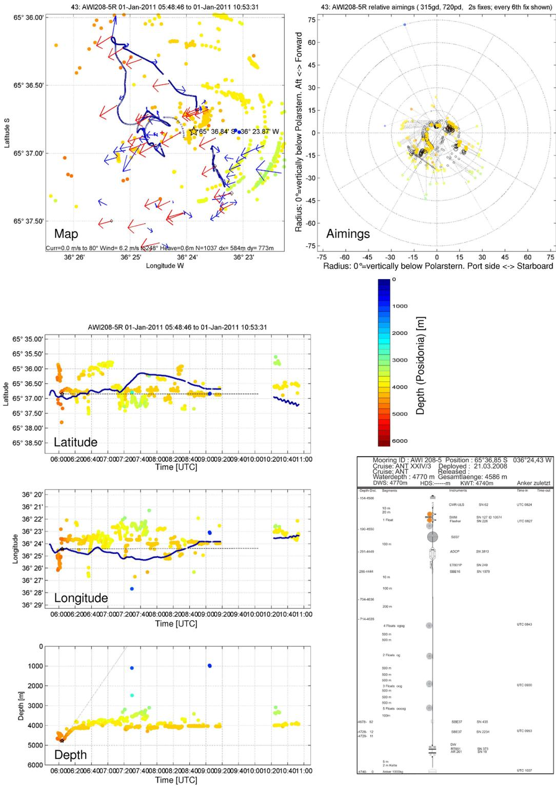
Mooring Recovery. Open Posidonia array used for extensive search when mooring was blocked below an ice floe.
