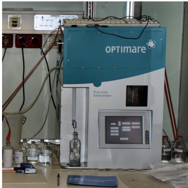
Fig. 3.1.2: Optimare Precision Salinometer (OPS)
