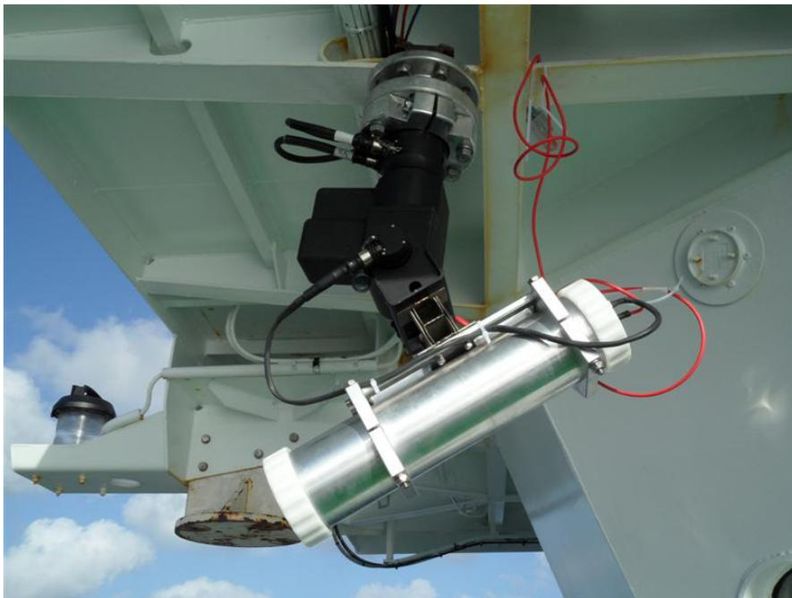
Fig. 13.1: The high-resolution camera in its metal housing mounted to the Pan-Tilt-Unit (PTU, black) installed on *Polarstern*'s crow's nest.
