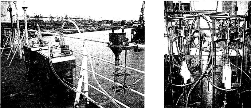
Fig. 6.1: High Volume Air Samplers at the observation deck and in-situ pumps attached to the sea water intake system of *Polarstern* for air and water sampling of PFC
