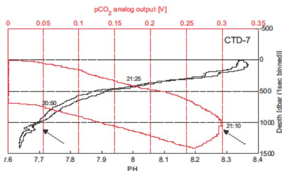
Fig. 6.19: Correlation between pH deviation and pCO<sub>2</sub> sensor response at 21:10 o'clock
