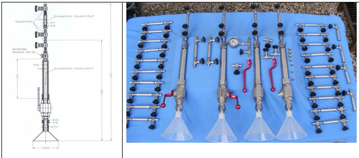
Fig. 5.3: Technical drawing of the pressure-retaining gas sampler and picture of the entire set of sampling and subsampling units
