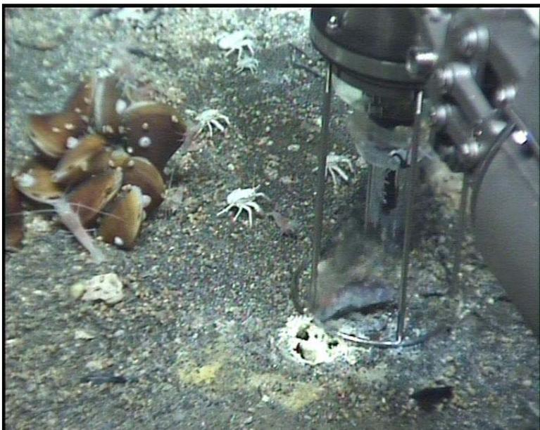
Fig. 5.2: The handheld is placed above a CO<sub>2</sub> vent to record temperature, pH, CO<sub>2</sub> and redox effects
