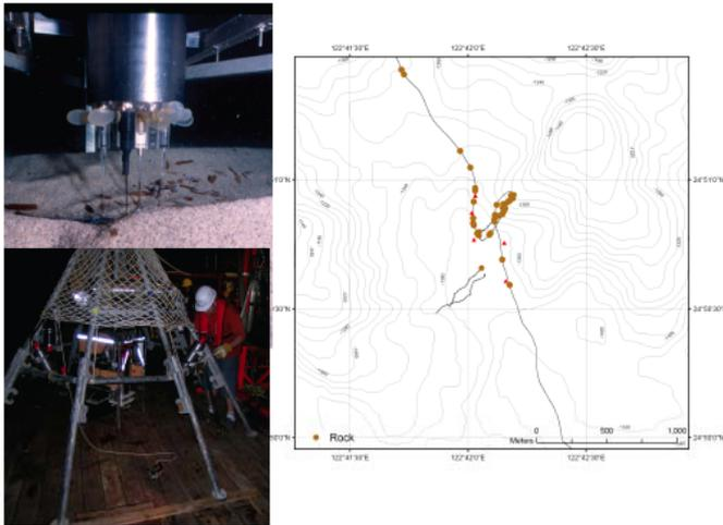
Fig. 6.35: Videoguided transects with the TV MUC (S-N) or ROV (SW-NE). A microprofiler was installed to measure CO<sub>2</sub> and pH during the visual monitoring of megafauna distribution
