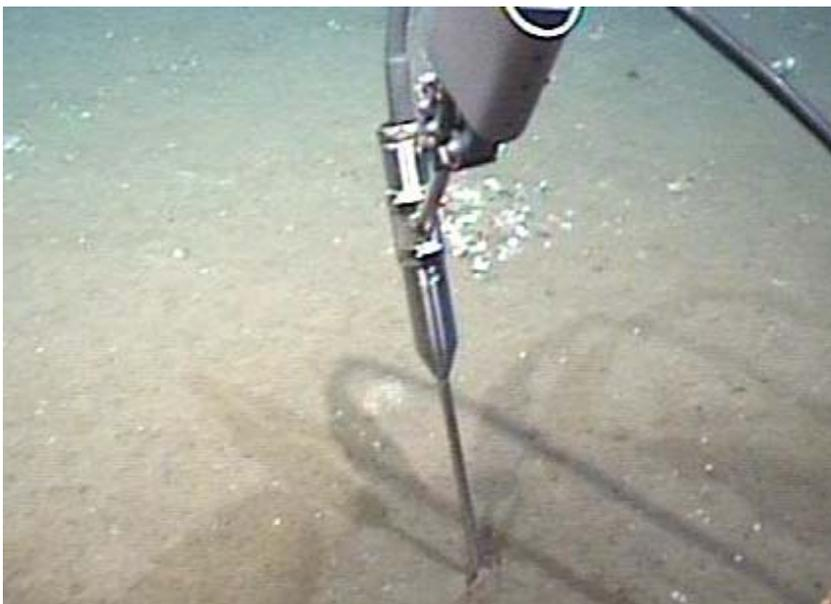
Fig. 5.4: ROV arm is pushing the T-lance into the sediment during dive 199-3
