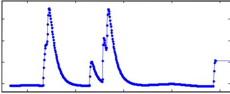
Fig. 6.18: Laboratory test time series of the *HydroC* data showing immediate signal increase due to breathing against the membrane
