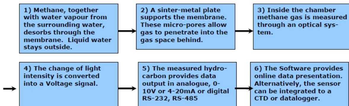
Fig. 5.7: Work flow of the *HYDOC-CH<sub>4</sub>* measuring process. The principle of this sequence remains the same for measuring CO<sub>2</sub> instead of methane
