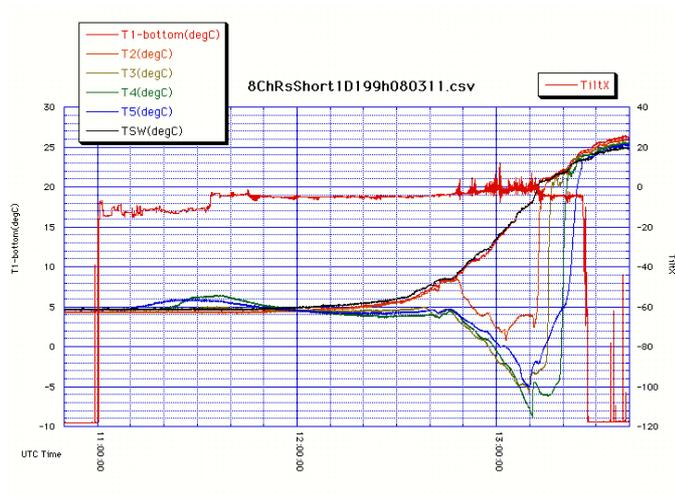
Fig. 6.38: Sampling, video observation on the front porch of the ROV during ascent, and T-record inside the CO<sub>2</sub>-capturing rod during ascent at the end of dive 199
