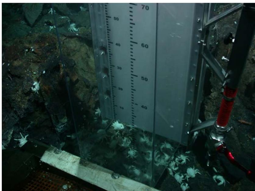
Fig. 5.6: Bubble imaging box at the seafloor above a CO<sub>2</sub>/CH<sub>4</sub> droplet emitting site. The front is positioned on the porch of the ROV, a gas sampler is attached on the right side of the frame
