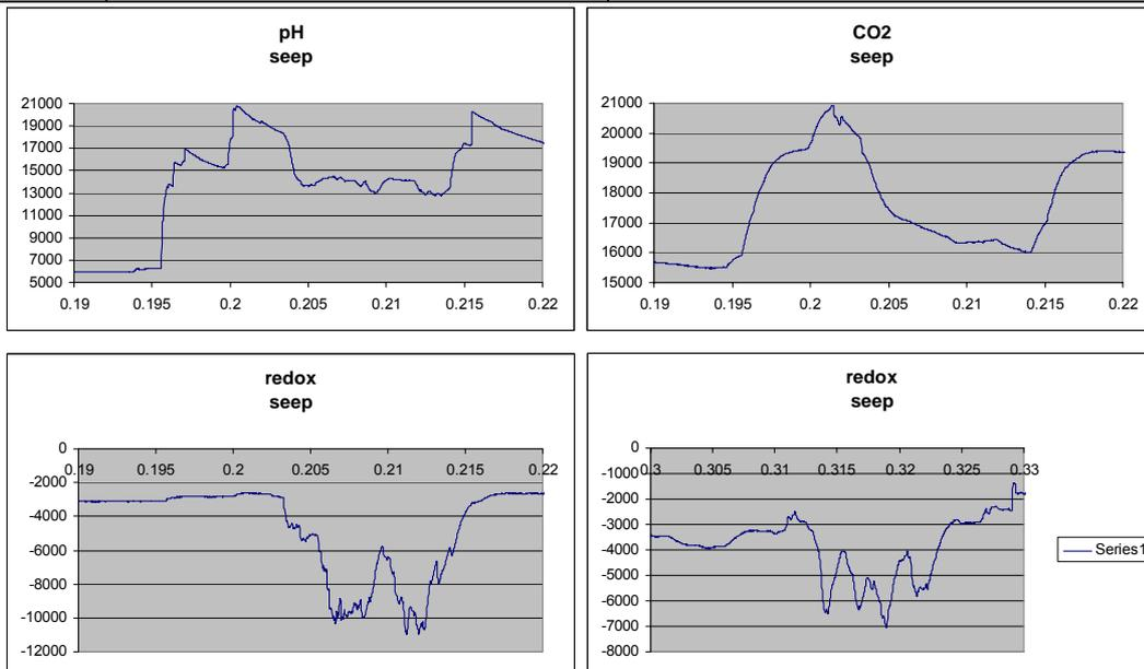
Fig. 6.20: Sensor measurements recorded above a CO<sub>2</sub> seep. pH signals increase with decreasing pH; CO<sub>2</sub> signals increase with increasing CO<sub>2</sub>, and redox signals decrease with decreasing redox state. The time is given as fraction of the day, normally the handheld was placed for ca 10 minutes
