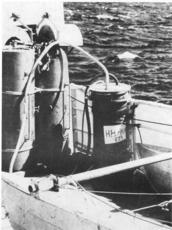
Fig. 3: Flow-through chamber of the continuous recording system. Sensors mounted inside the chamber are: temperature-sensor (T1), conductivity (L1), fluorescence of Chl.a (F1) and pressure (P1) (physical dimensions of the sensors are similar to those shown in Fig. 2).
