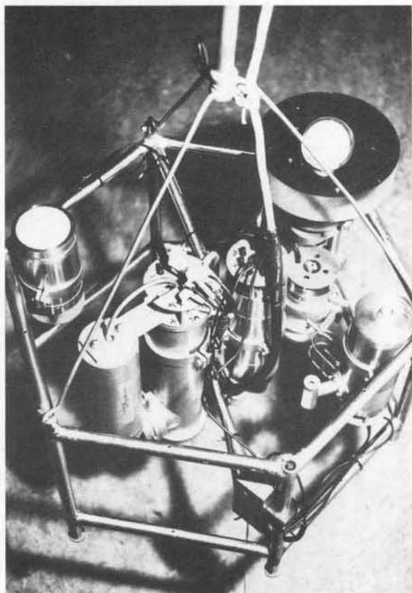
Fig. 2a) Rack I with sensors measuring the selective optical density ( $D_{670}$ ) and the fluorescence of Chl.a (FS), the central underwater unit, sensors measuring the downwelling scalar irradiance ( $E_{od}$ ), the upwelling scalar irradiance ( $E_{ou}$ ) and depth (P2), temperature (T2), conductivity (L2) (from left to right).
