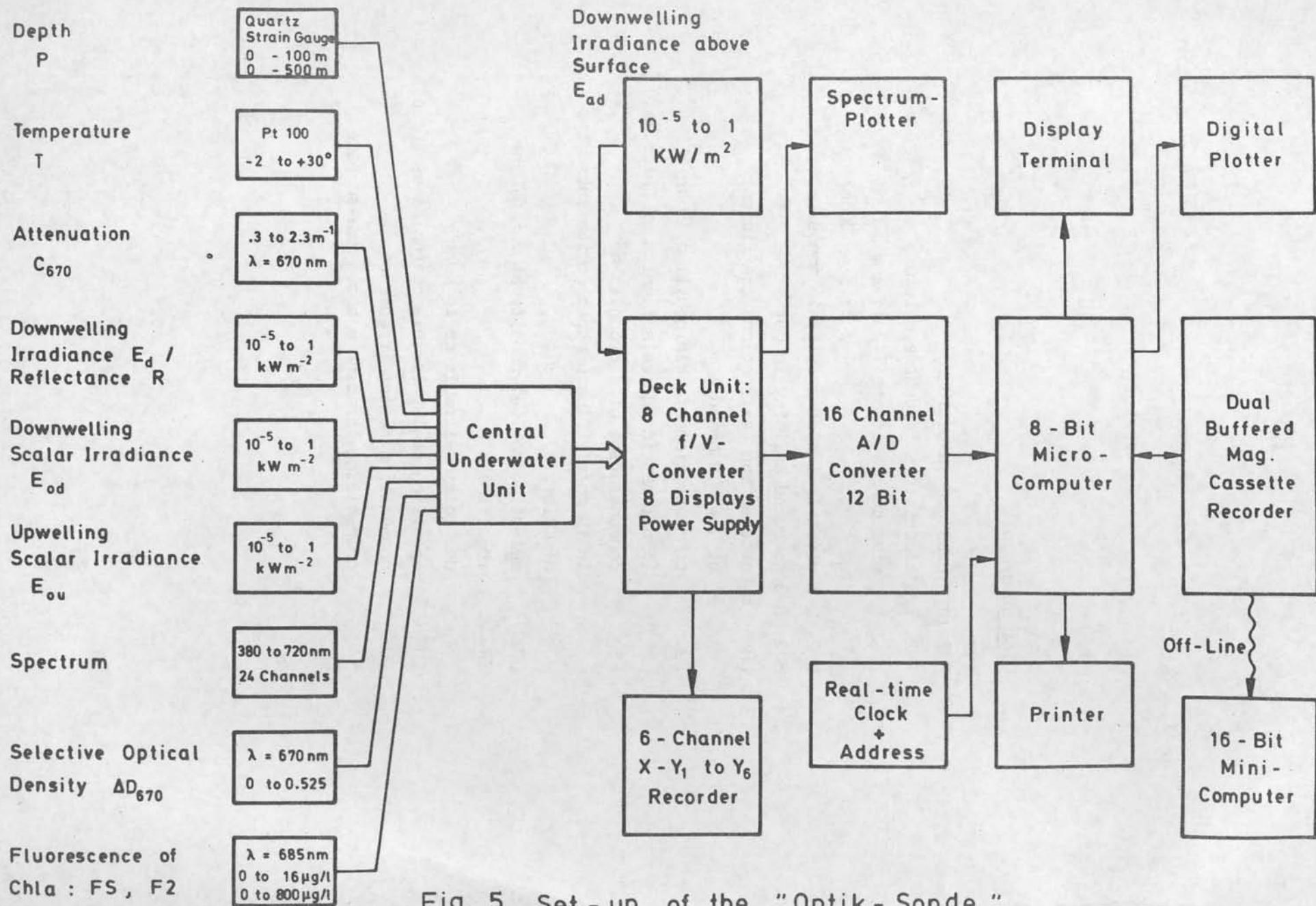
Fig. 5 Set-up of the "Optik-Sonde" profiling measuring system
