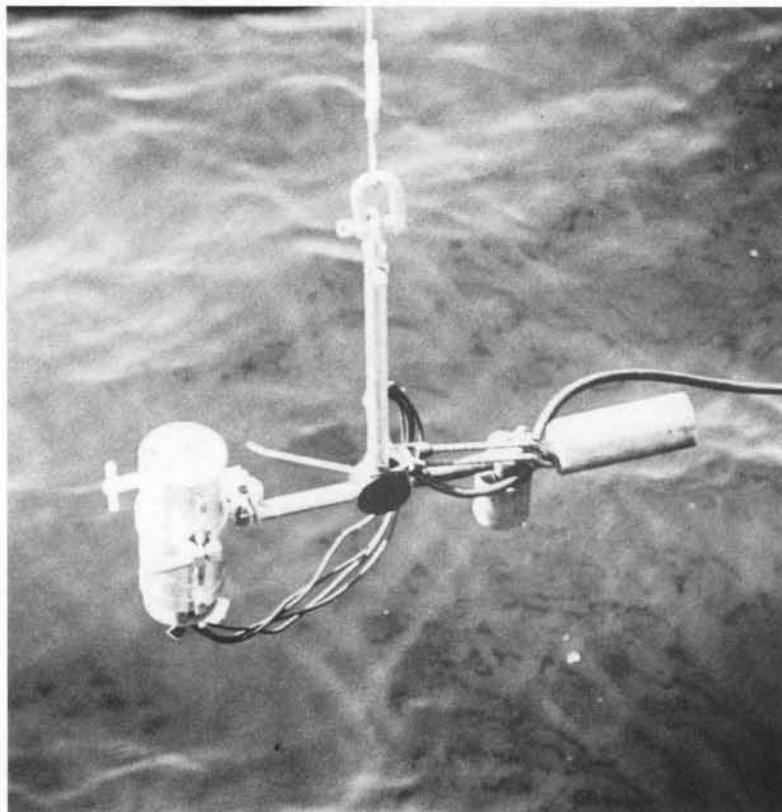
Fig. 4: The 24-channel spectroradiometer, in this alignment, for the determination of the spectrum of the downwelling irradiance
