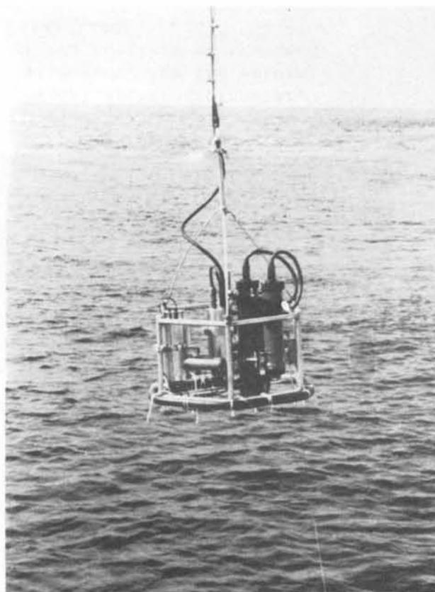
Fig. 2b) Rack II with sensors measuring the attenuation coefficient of light (CR), the downwelling irradiance ( $E_d$ ), the diffuse reflectance (R), the fluorescence of Chl.a (F2) and depth (P3), temperature (T3), conductivity (L3).
