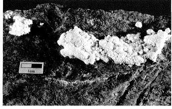
Fig. 2: Sample KB 102 from northern Heimefrontfjella, an augen gneiss with firmly attached salt crust.
