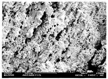
**Fig. 4:** a) Pore radii distribution of calcite crust B22.2.94 from southern Heimefrontfjella. b) SEM image of B22.2.94 in profile (lower margin parallel to rock surface), showing a coarse-grained layer with oblique channel-like pores.
