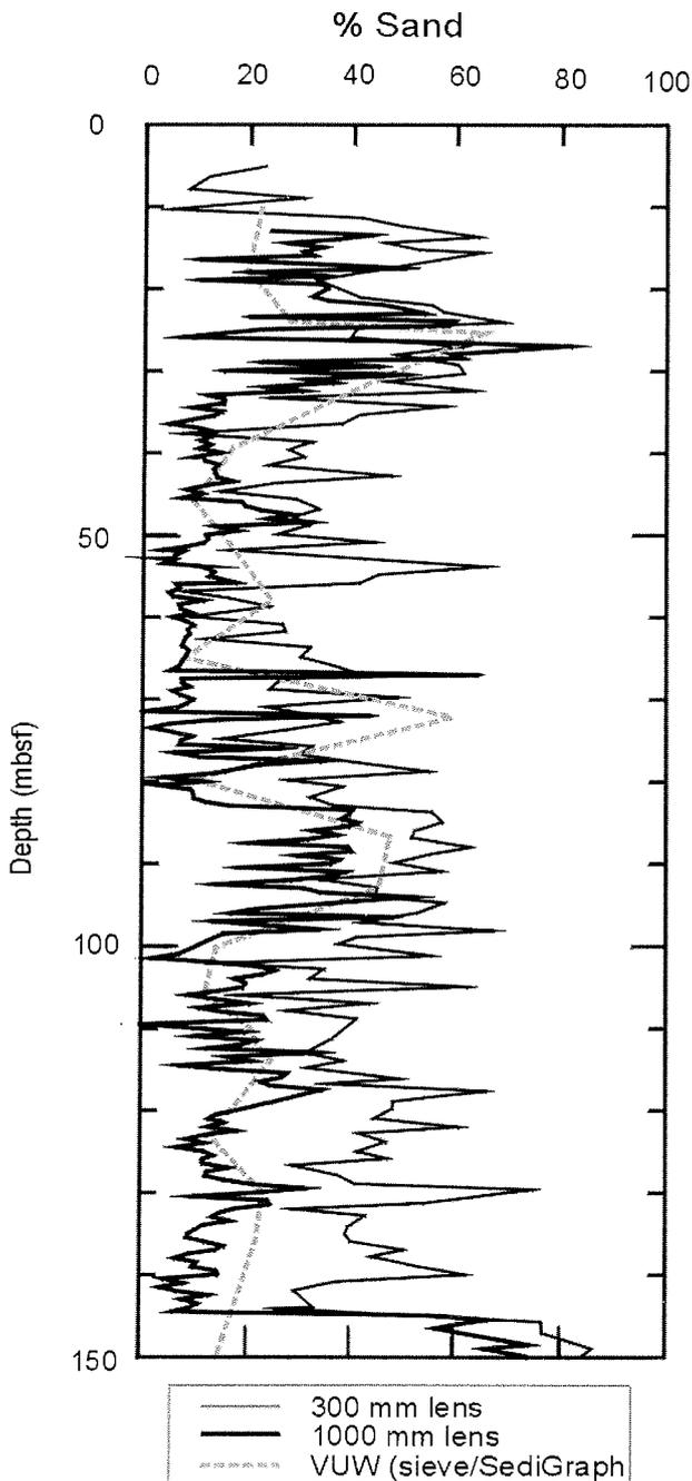
Fig. 2 - Comparison of percent sand (<1000  $\mu\text{m}$ ) estimates derived from analyses performed on 300 and 1000 mm focal length lenses with measurement ranges of 0.5 - 600 and 1.8-2000  $\mu\text{m}$  respectively. Note that because different lenses have different size class limits, "sand" is considered to be material coarser than 56  $\mu\text{m}$  and 60  $\mu\text{m}$  for the 300 and 1000 mm lenses, respectively.
